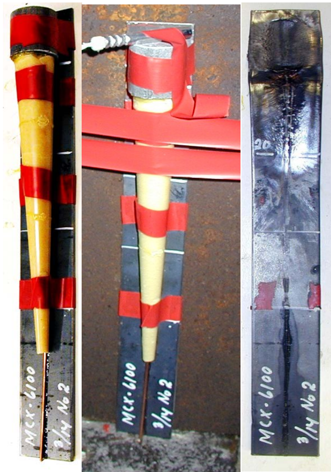
Figure 3.3 Pictures of test item, setup and witness plate for conical charge No 3 after firing (right).
