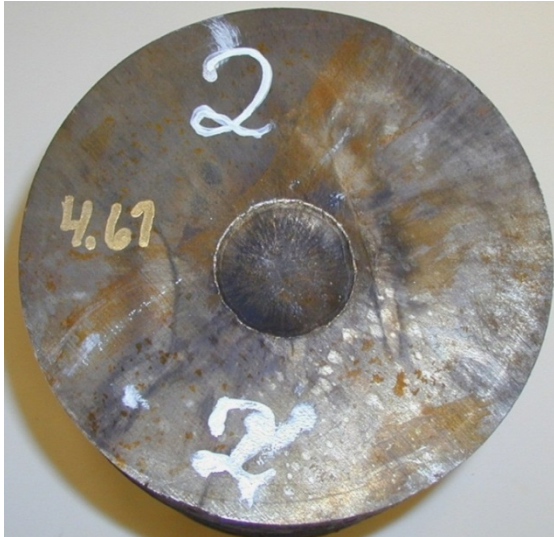
Figure 3.25 Picture of the Dent plate after firing of MCX-6100 CH 6079/13 charge No 8.
