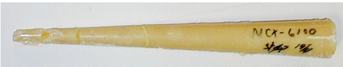
Figure 2.9 Conical charge No 5 cast 19/14 after it was released from the mould.
