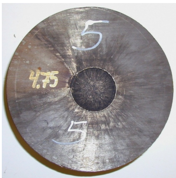
Figure 3.28 Picture of the Dent plate after firing of MCX-6100 CH 6079/13 charge No 3.
