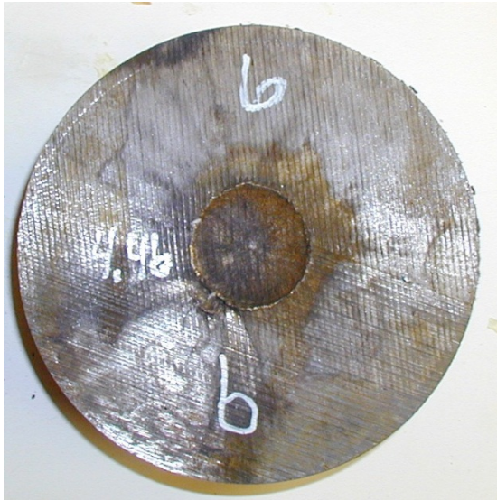
Figure 3.29 Picture of the Dent plate after firing of MCX-6100 CH 6079/13 charge No 5.
