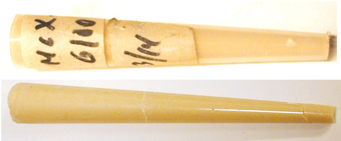
Figure 2.4 Conical charge before and after it was released from the mould.
