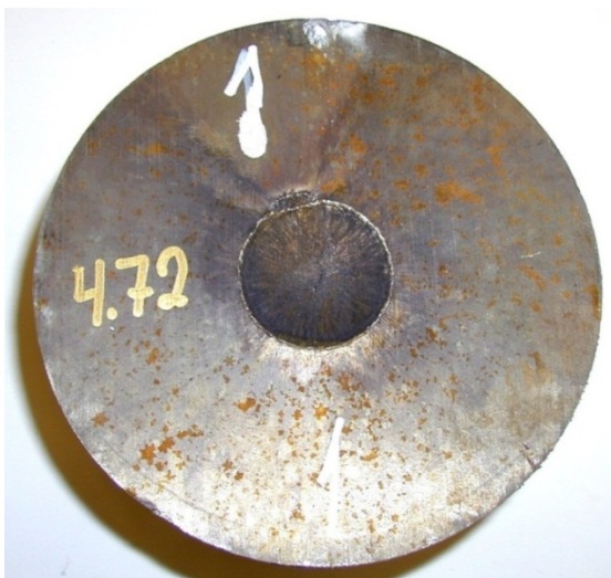
Figure 3.24 Picture of the Dent plate after firing of MCX-6100 CH 6079/13 charge No 1.
