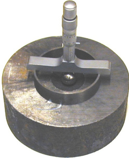
Figure 2.12 Picture of the tool used to measure the Dent depth.
