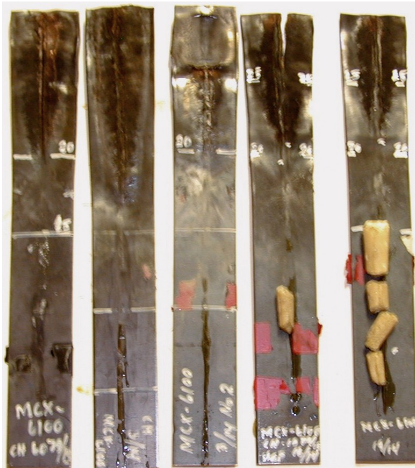
Figure 3.6 Witness plates for the five performed tests for determination of the critical diameter of MCX-6100 CH 6079/13.
