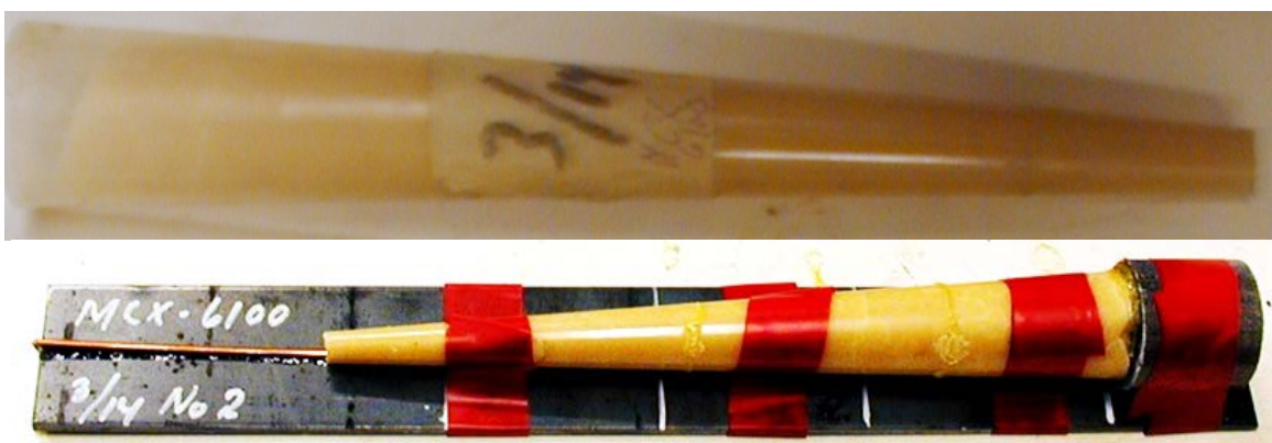
Figure 2.6 Test item in the mould (top) and on the witness plate with attached booster (bottom).
