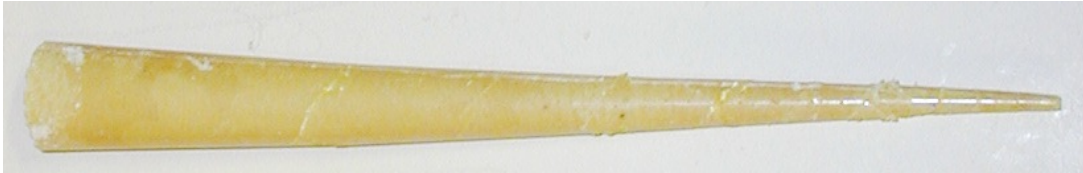
Figure 2.7 Picture of conical charge No 4 after it was taken out of the mould.
