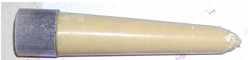
Figure 2.3 Picture of the first conical charge after the booster had been glued to the top.
