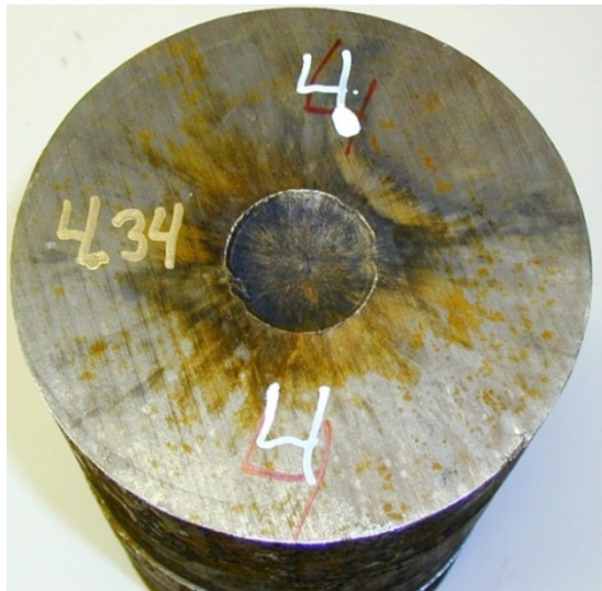
Figure 3.27 Picture of the Dent plate after firing of MCX-6100 CH 6079/13 charge No 7.
