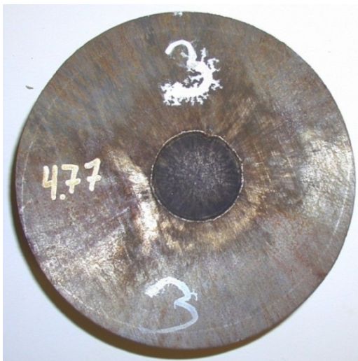
Figure 3.26 Picture of the Dent plate after firing of MCX-6100 CH 6079/13 charge No 3.
