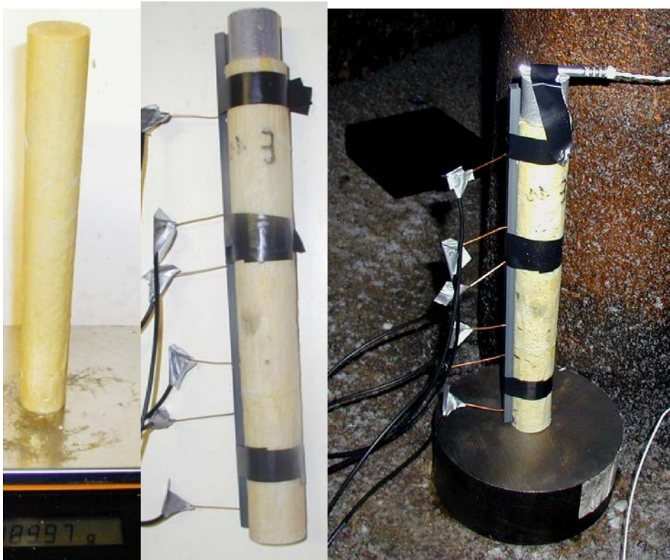
Figure 3.16 The figure shows at left the original charge, in the middle the test item after being assembled with ionization pins and to the right the test setup for the firing.
