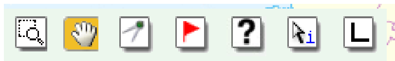
Figure 4.5 Controls in bottom left corner. From left: zoom in, pan, put waypoints/markers on the map, click controls for help, information on map features ('i'-button), sound propagation model (Lybin).
