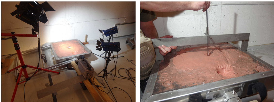
(a) The experimental set-up after a ball drop test. The steel ball is seen in the middle of the clay. (b) The crater depth is measured with a calliper with the frame as reference after an ball drop test.
