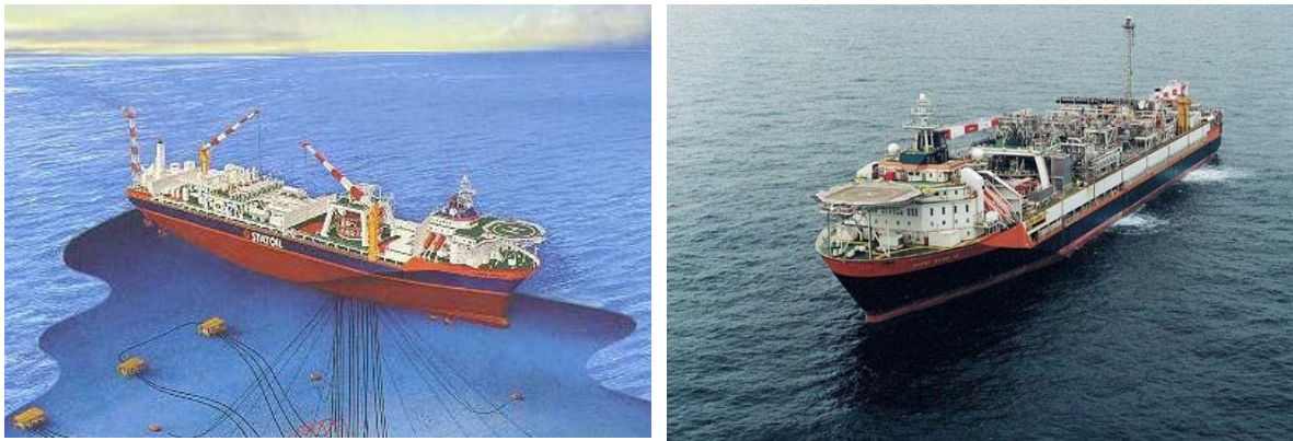
Figure 3.1 Illustration and image of the oil production vessel Norne FPSO. Source: Statoil
