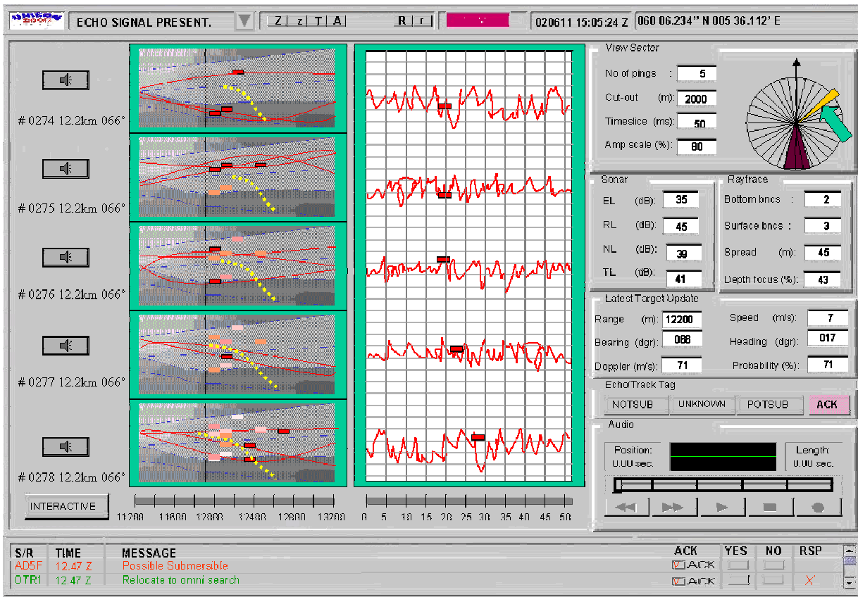
Figure 5.2 The illustration shows a possible solution for an echo signal structure classifier. Buttons on the left activate the sound of the time slice of the respective ping. Going to the right, a perspective view of the area selected for analysis is shown including the raytrace and echo positions. In the centre, the time series signal is drawn of the matched filter output for the section selected by the operator. Again, on the top right, a widget showing the angle of view is included. Further down, some data showing the hydro-acoustic model estimations are shown which may tell the operator something about the trustworthiness of the signal. Below this, there is again a dialogue for the operator to make any contribution to the tagging of an echo or track. On the bottom right there is an audio operation dialogue.
