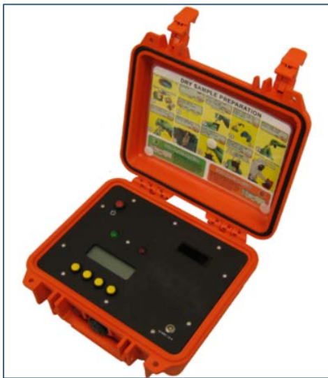
Figure 4.2 The QTL Biosensor 2200 R handheld bio-detection instrument.
