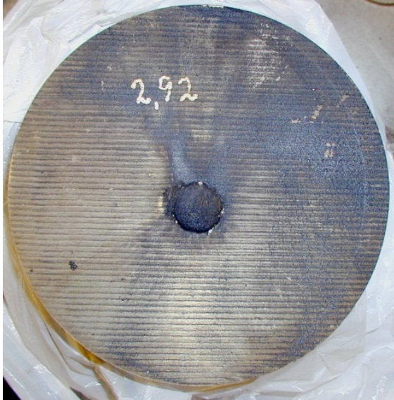
Figure 3.38 Picture of the Dent witness plate for the test item of composition Sats-230/13.
