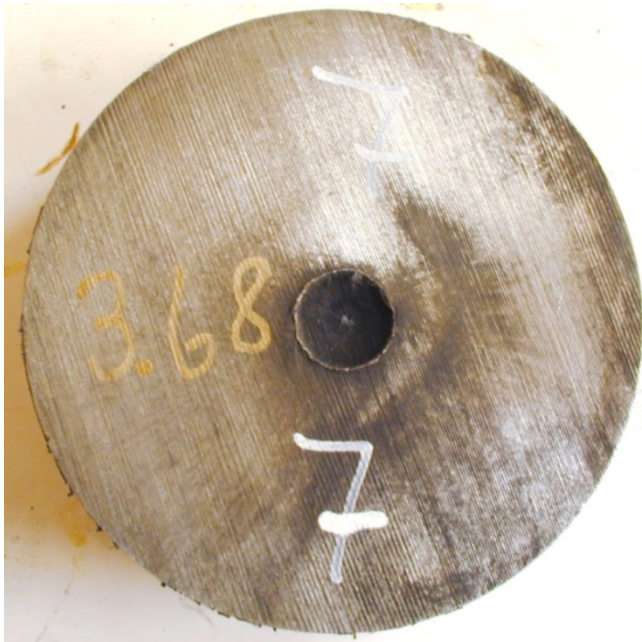
Figure 3.49 The witness plate from firing No 7 with a test item of Sats-400/13.
