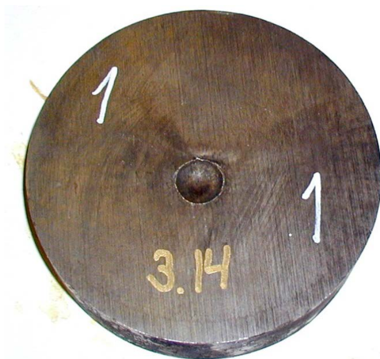
Figure 3.42 The witness plate from firing No 1 with a test item of Sats-432/13.
