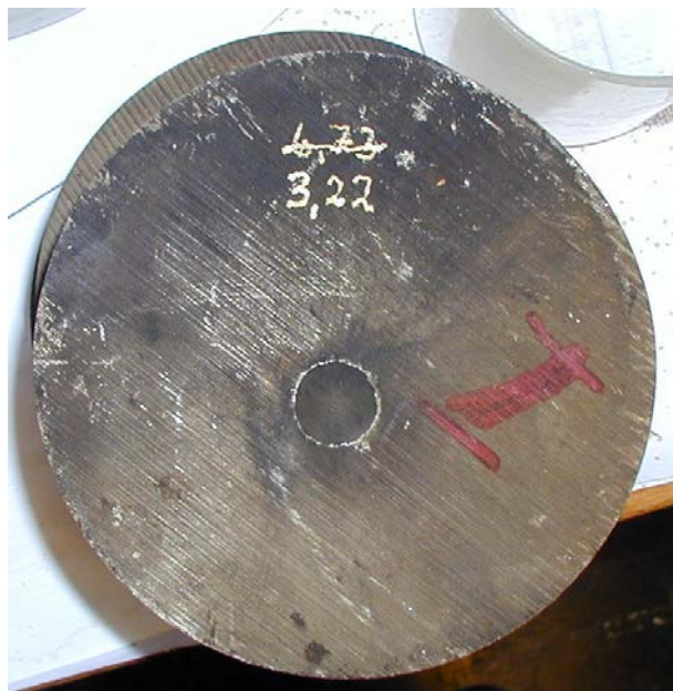
Figure 3.40 The Figure shows a picture of the witness plate from firing No 2 with a test item containing composition Sats-258/13.
