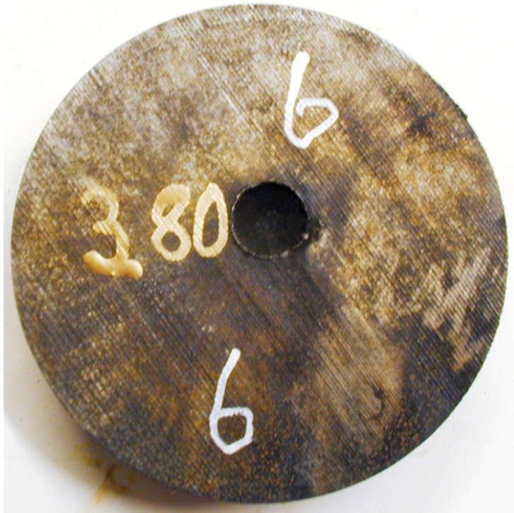
Figure 3.46 The witness plate from firing No 6 with Sats-430/13.
