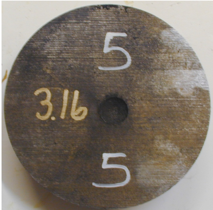
Figure 3.48 The witness plate from firing No 5 with a test item of Sats-400/13.
