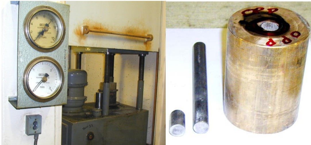
Figure 2.1 Pictures of applied press and tool for initial press study of composition Sats-258/13.
