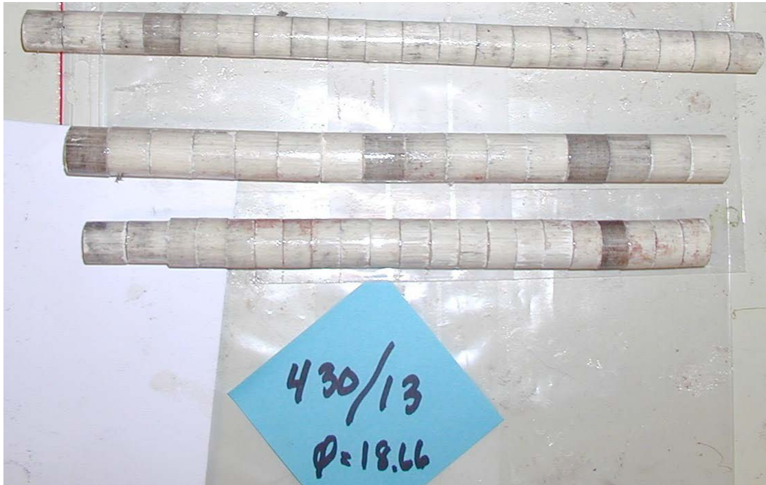
Figure 2.5 Picture of Sats-430/13 pellets after being glued together to three test items for determination of detonation velocity and detonation pressure.
