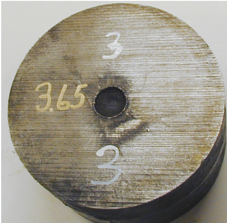
Figure 3.44 The witness plate from firing No 3 with a test item of Sats-432/13.
