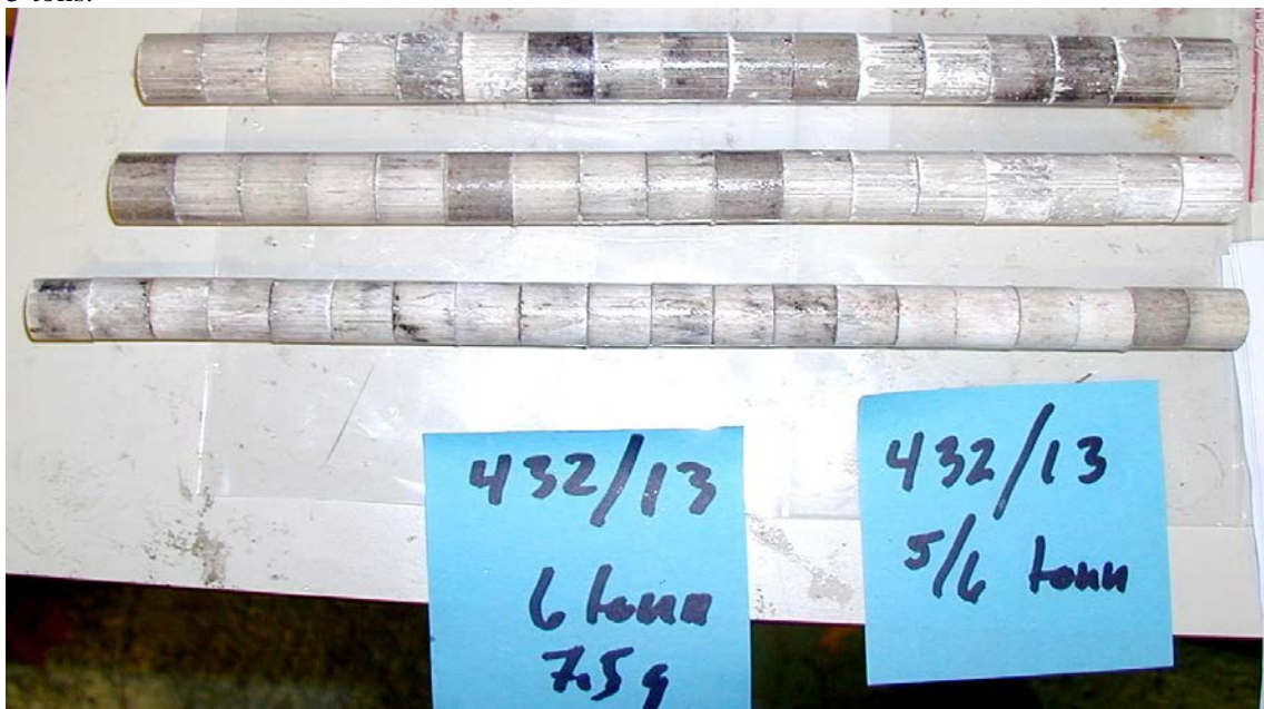
Figure 2.6 Picture of Sats-432/13 pellets after they have been glued together to three test items for determination of detonation velocity and pressure.
