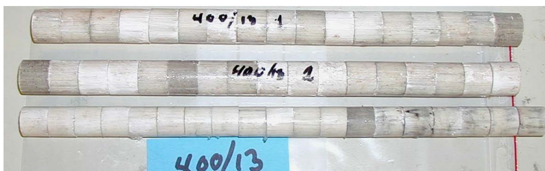
Figure 2.4 Picture of Sats-400/13 pellets after they were glued together to three test items for determination of detonation velocity and pressure.
