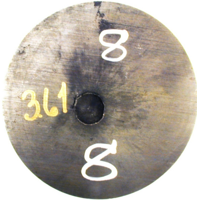
Figure 3.47 The witness plate from firing No 8 with a test item of Sats-430/13.
