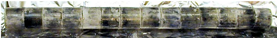
Figure 3.5 The pellets of Sats-258/13 after been glued together to a test item.
