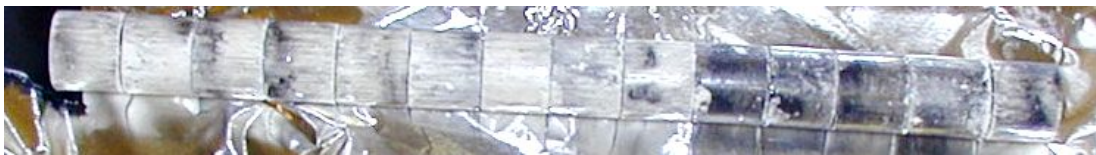
Figure 3.1 The figure shows the test charge after being glued together.
