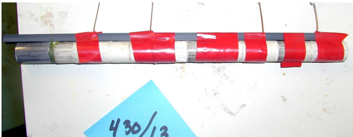
Figure 3.23 The figure shows the positions of the ionization pins.
