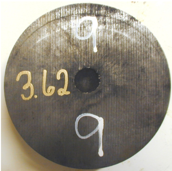
Figure 3.50 The witness plate from firing No 9 with a test item of Sats-400/13.
