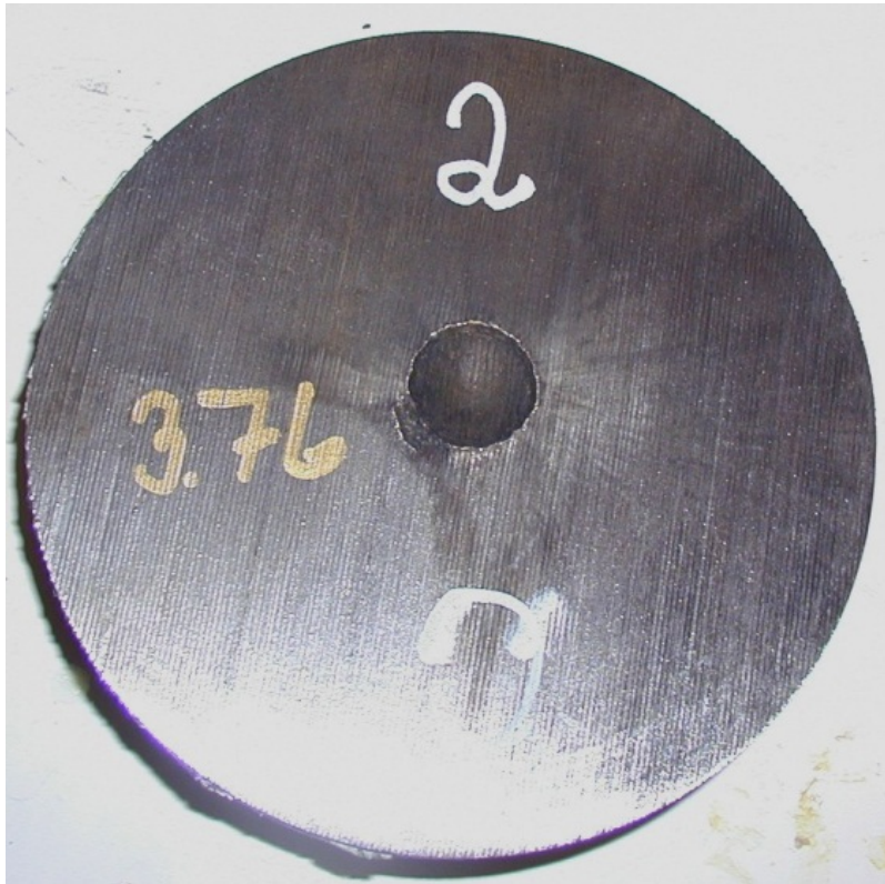
Figure 3.43 The witness plate from firing No 2 with a test item of Sats-432/13.
