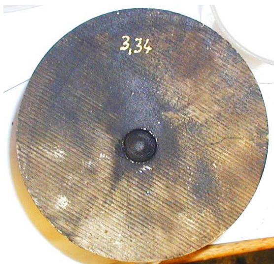
Figure 3.41 Dent witness plate from firing No 3 with a test item of composition Sats-258/13.
