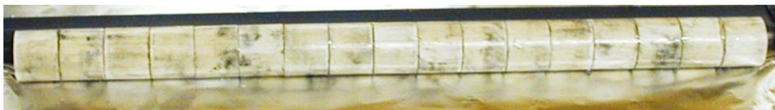
Figure 3.9 Pellets of Sats-258/13 after being glued together to be test item No 3.
