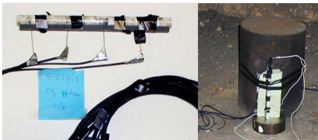
Figure 3.7 Pictures of the test item after the ionization pins were added, to the left, and test setup for firing No 2 with Sats-258/13 to the right.
