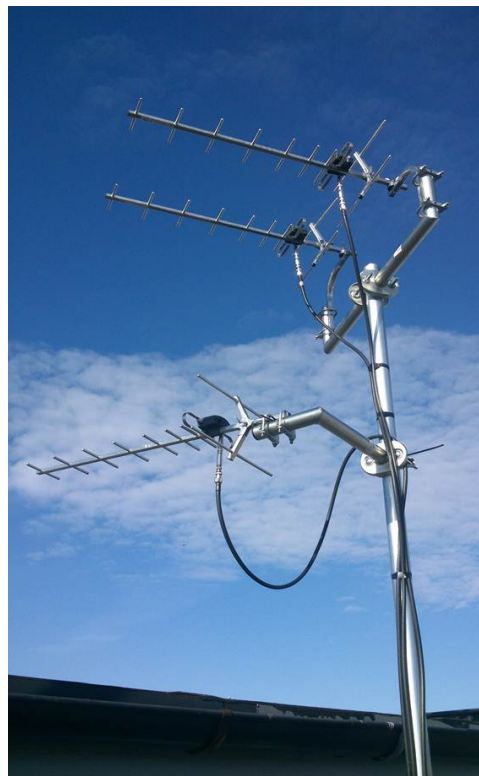
Figure 2.1 A picture of the radar receiver antennas with the surveillance antennas on top and the reference antenna below.
