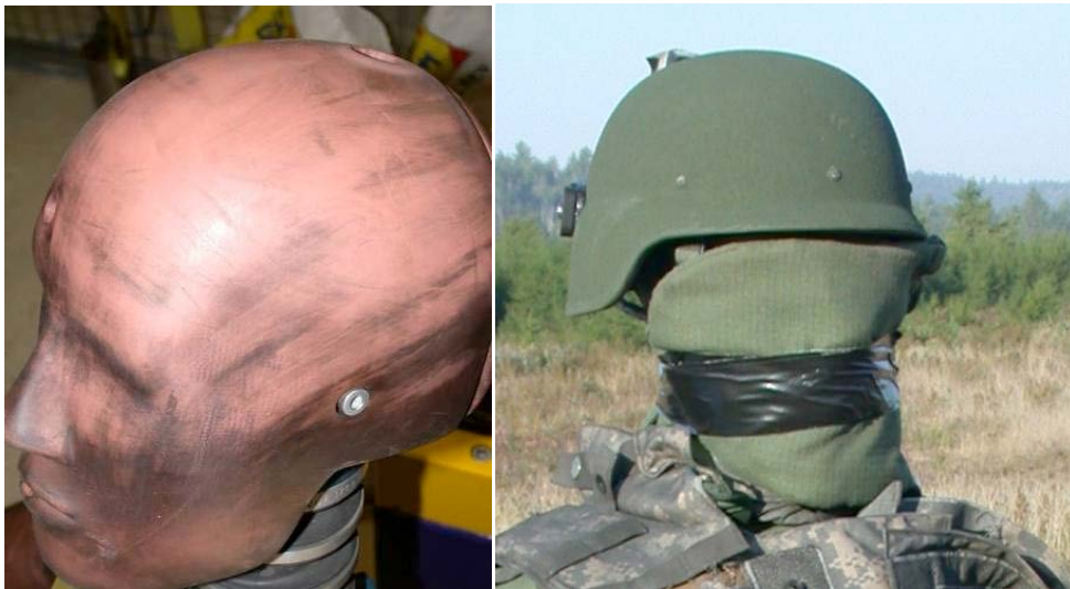
Figure 2.1 Hybrid III dummy with and without helmet. (Pictures from [5]).
