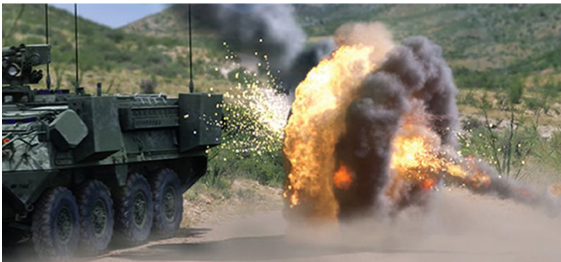
Figure 2.1 The hard-kill active protection system Quick Kill from Raytheon intercepting and destroying an incoming projectile (Raytheon).
