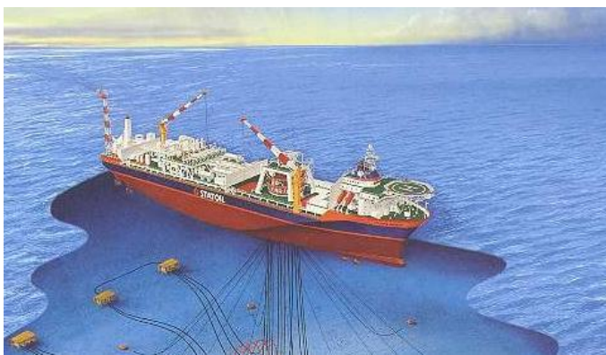
Figure 5.1 Illustration of the oil production vessel Norne FPSO. ©Statoil
