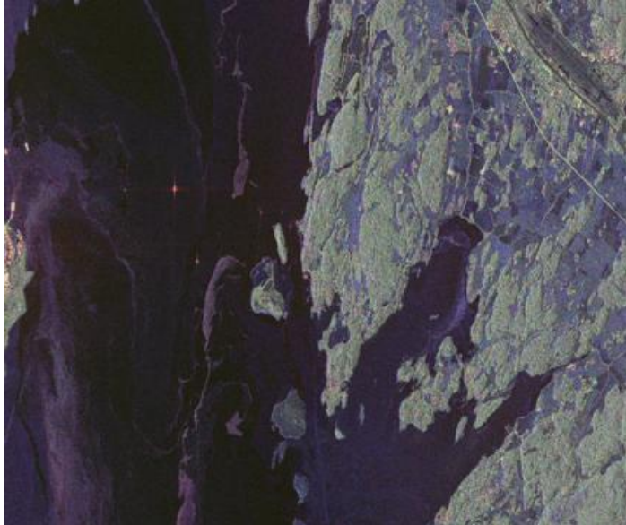
Figure 4.1 Segment of a RADARSAT-2 Standard Quad-Pol mode image on February 7 th 2010 from the Oslofjord. The four different polarisation channels have been combined using the Pauli decomposition method.
