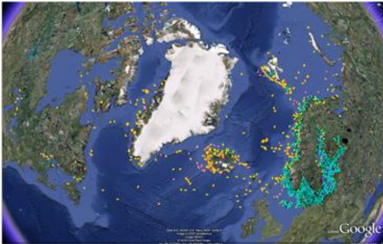
Figure 6.4 The first AIS data from AISSat-1. The yellow and orange symbols show the new AIS data that the satellite gives in addition to the data from the land-based network shown in turquoise symbols.
