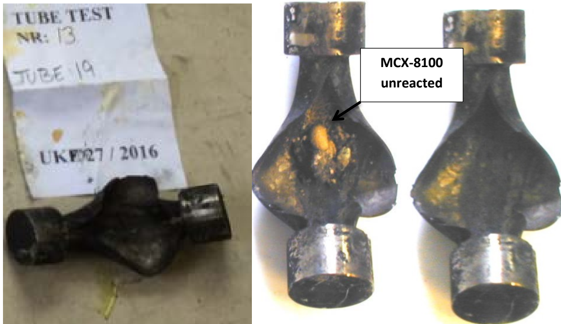
Figure 3.12 Pictures of the recovered tube after testing.
