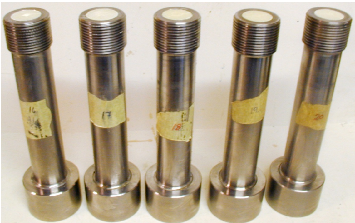
Figure 2.3 Picture of tubes No 16 to No 20 after cleaning and modification of the end surfaces.
