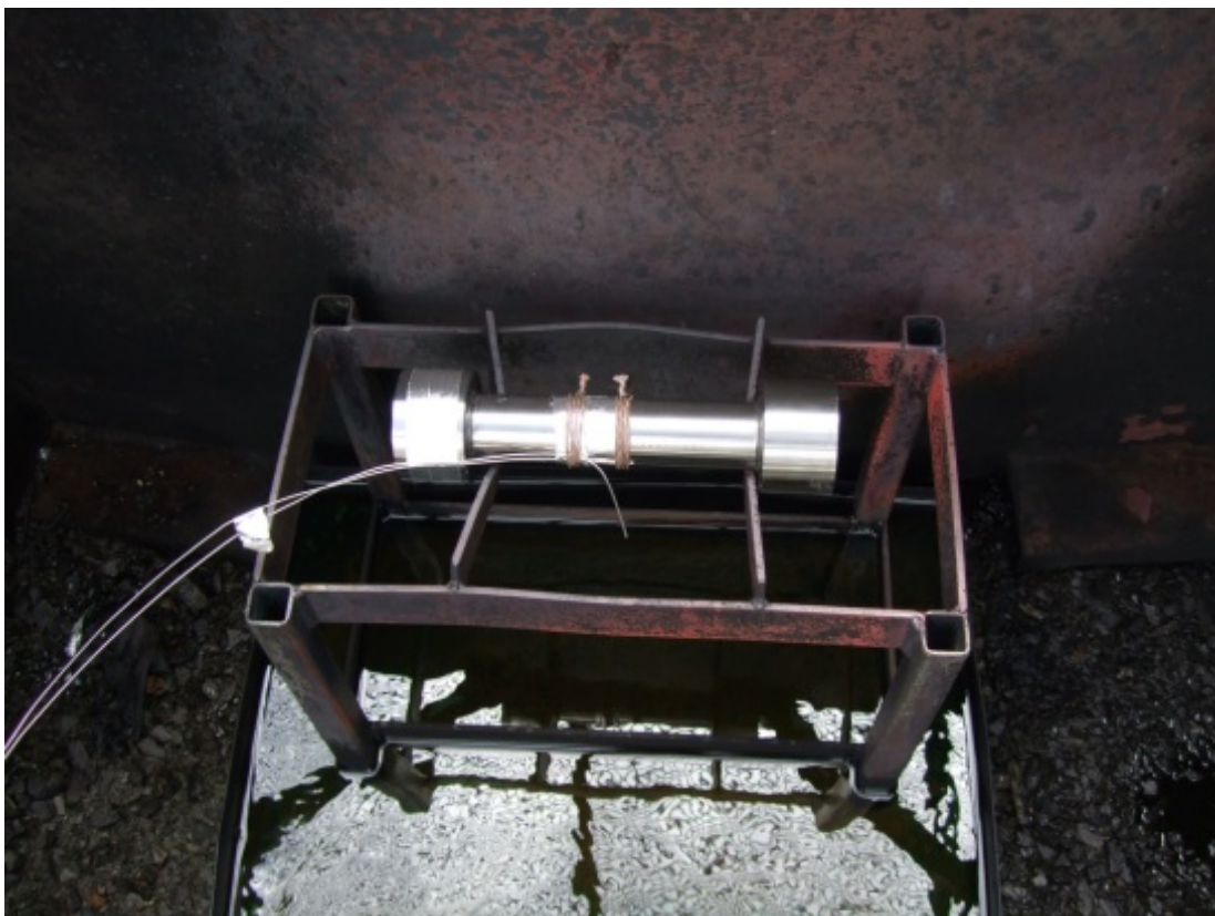
Figure 2.8 Picture of test item with the two thermocouples seen from above.
