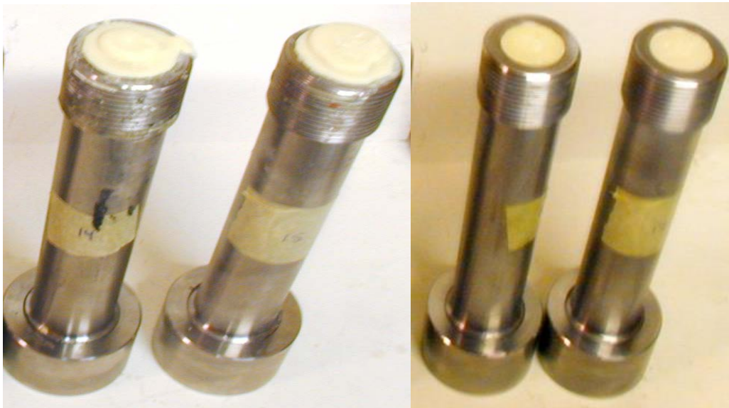
Figure 2.1 Tubes No 14 and No 15 as received from Chemring Nobel AS, left picture. Right picture shows the tubes after cleaning and modification of the end surfaces.
