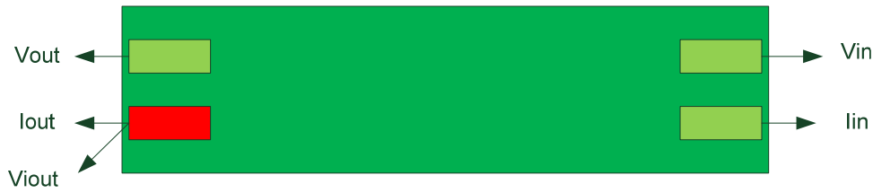
Figure 4.1 Principle for measuring contact resistance on the red pad.
