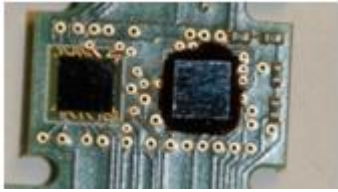
Figure 10.7 Test device (to the right) with underfill before firing.
