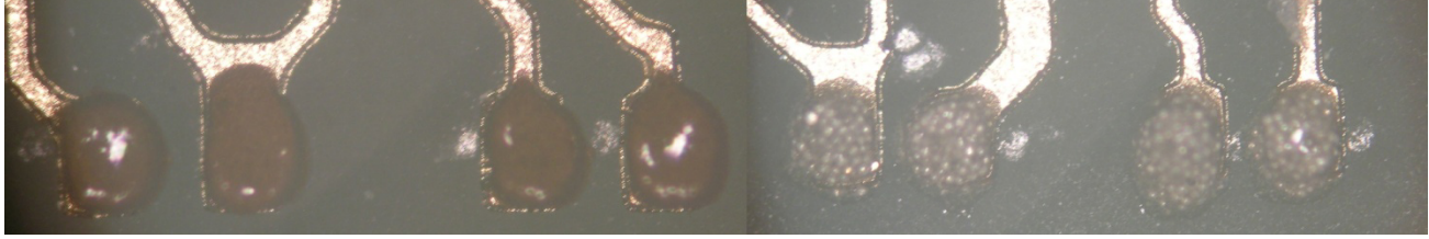
Figure 6. Picture showing stencil printing of ICA-B (left) and ICA-A (right) onto the firing boards (I1-I8).
