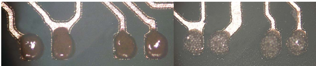
Fig. 6 Picture showing stencil printing of ICA-B (left) and ICA-A (right) onto the firing boards (I1 through I8).
