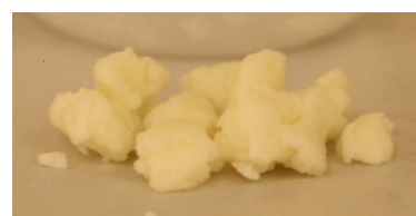
Figure 1: Non-uniform suspension of adhesive filled with 60 volume% of SPP
