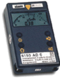
Figur 2.1 Automess modell 6150 AD radiologisk sensor. (Foto: Automess).
