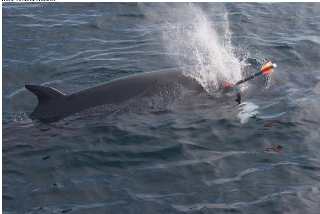
Figure 4.18. Successful deployment of CTAG to a Minke whale despite the tag hitting the water in front of the animal. The carrier seen detaches upon impact leaving only the small tag on the whale.
