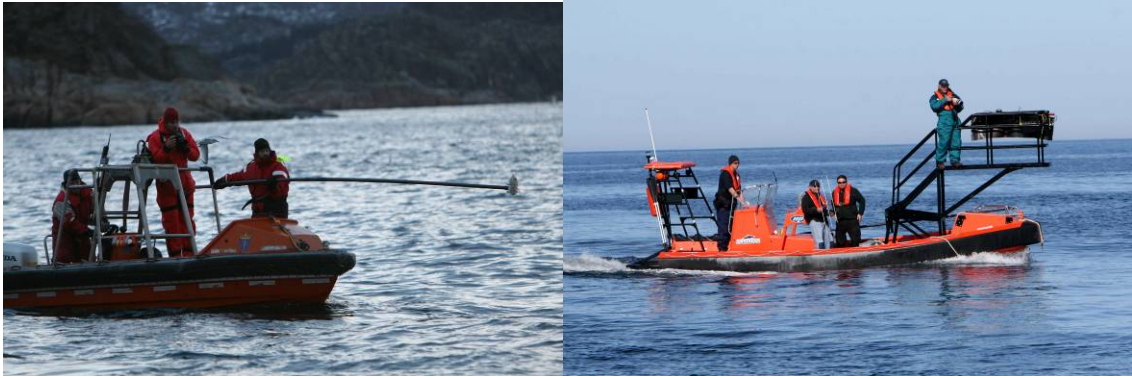
Tag boat 1 (left) and Tag boat 2 (right). The lifting arrangement on Tag boat 1 will be modified to enable us to pick it up with the David crane. Tag boat 2 will be modified with a 2 person elevated MMO-station behind the driver.
