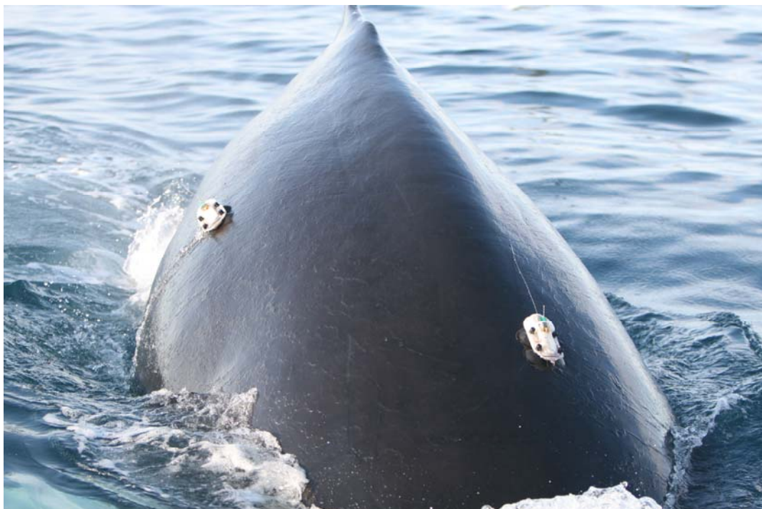
Figure 4.4. Humpback whale tagged with two DTAGs to improve VHF tracking capability, and to increase the chance that at least one DTAG stays on for the entire duration of the experiment (16 hrs). The DTAGs both have an extra GPS-tag attached to them.
