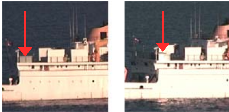
Figure 6.42 Images of the two grey test panels from DRDC-V mounted on the starboard side of CFMV Quest, illuminated by sun. In the image to the right there is specular reflection, especially from the panel to the left, SIMVEX run 33C
