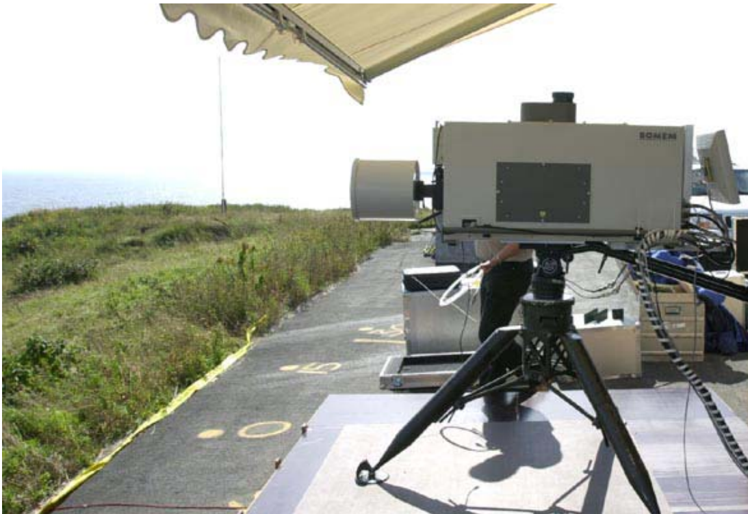
Figure 3.2 The Bomem DA5 Spectroradiometer in position for measurement on the platform outside the container
