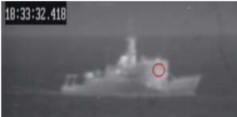
Figure 6.29 Milcam IR image from a day run, measuring the sun illuminated front of the bridge, SIMVEX run 18
