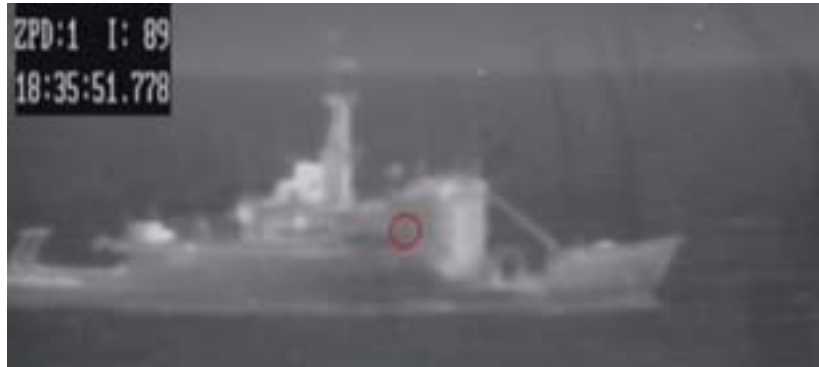
Figure 6.12 Milcam IR image from a day run, measuring the shaded starboard side of the bridge, SIMVEX run 18
