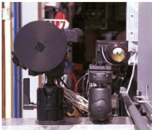
Figure 3.4 The Amber Sentinel and Inframetrics Milcam IR cameras
