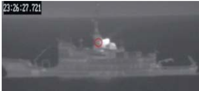
Figure 6.9 Milcam IR image from a night run, measuring the port side of the funnel, SIMVEX run 26
