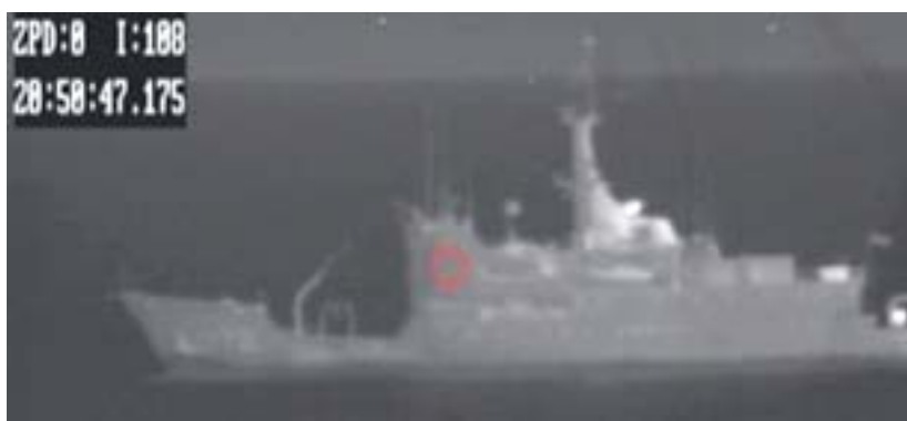
Figure 6.20 Milcam IR image from a day run, measuring the sun illuminated port side of the bridge, SIMVEX run 32
