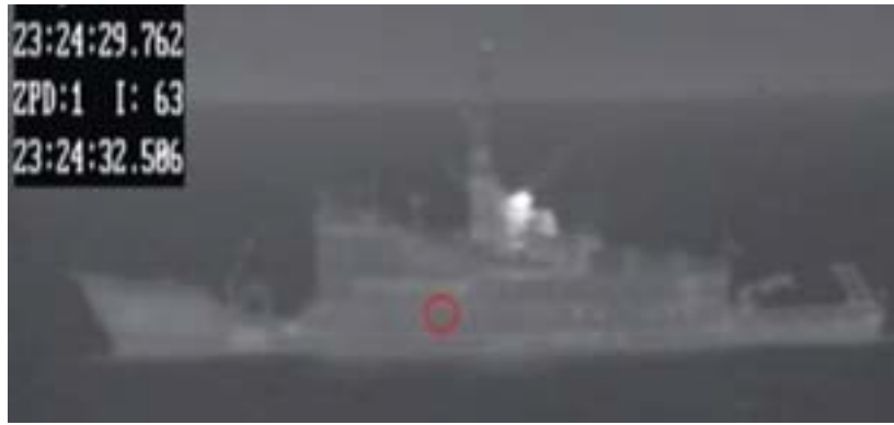
Figure 6.5 Milcam IR image from a night run, measuring the port side of the hull, SIMVEX run 26
