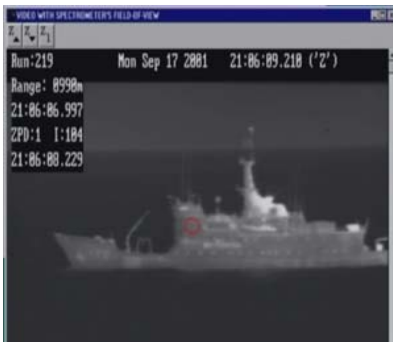
Figure 3.5 Output video image from the Matrox 4sight unit, showing the Milcam IR image with the FTIR field of view (red circle), plus additional text information
