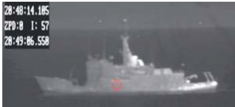
Figure 6.31 Milcam IR image from a day run, measuring the sun illuminated port side of the hull, SIMVEX run 32
