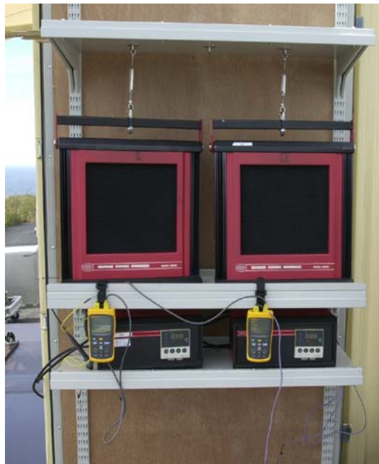
Figure 3.3 The two blackbodies mounted on the container door for FTIR reference measurements
