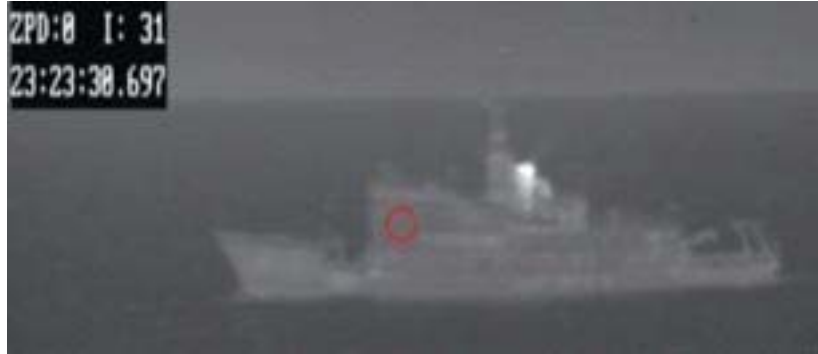
Figure 6.7 Milcam IR image from a night run, measuring the front of the bridge, SIMVEX run 26
