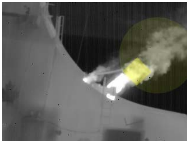
Figure 7.7 IR image taken by NRL with the Indigo Merlin camera installed on helicopter. The opaque, yellow circle embedded in the image represents the size of the FTIR Spectroradiometer's field of view, while the brighter square represents the estimated size of the area used in our plume model, SIMVEX run 23B
