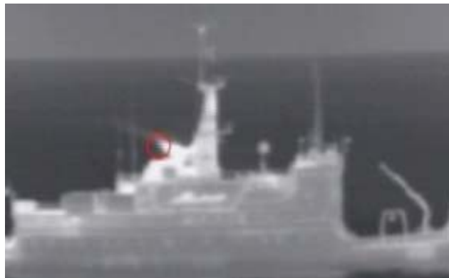
Figure 7.1 Milcam IR image from a measurement of the ship plume, SIMVEX run 23B
