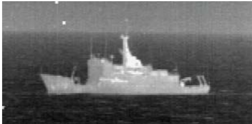
Figure 6.25 Sentinel IR image from a day run, showing the sun illuminated port side and the shaded front of the ship, SIMVEX run 19
