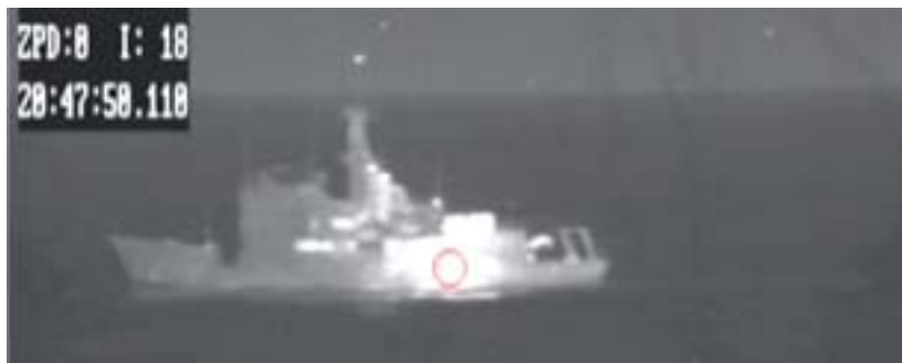
Figure 6.38 Milcam IR image (3-5 \mu\text{m} ) from a day run, measuring specular sun reflection from the port side of the hull, SIMVEX run 32
