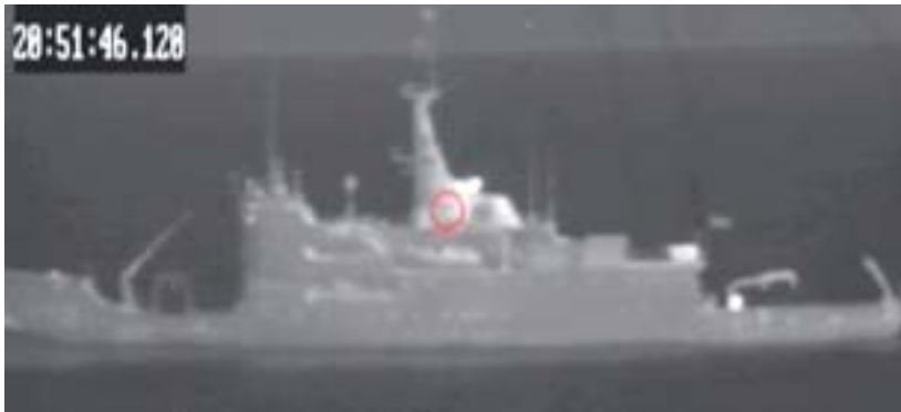
Figure 6.34 Milcam IR image from a day run, measuring the sun illuminated port side of the funnel, SIMVEX run 32
