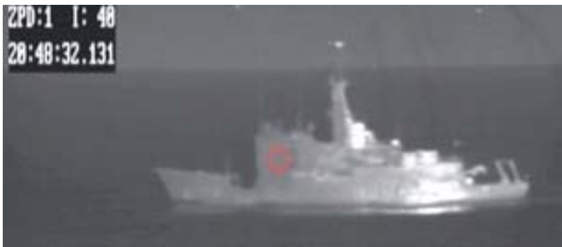
Figure 6.15 Milcam IR image from a day run, measuring the shaded front of the bridge, SIMVEX run 32
