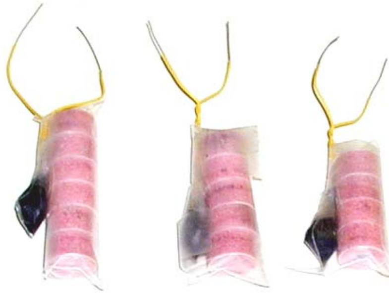
Figure 3.45 Picture of how the high density pellets of PETN were packed for testing in the Closed Vessel.
