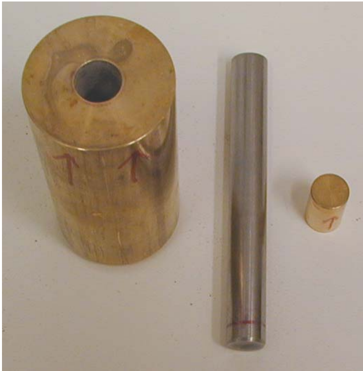
Figure 2.2 Picture of the press tool used to produce pellets of moderate density.
