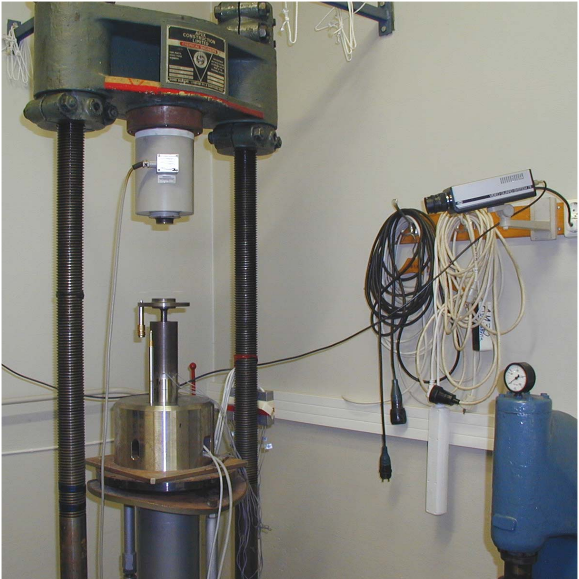
Figure 2.3 Picture of press and press tool used for production of high-density pellets.
