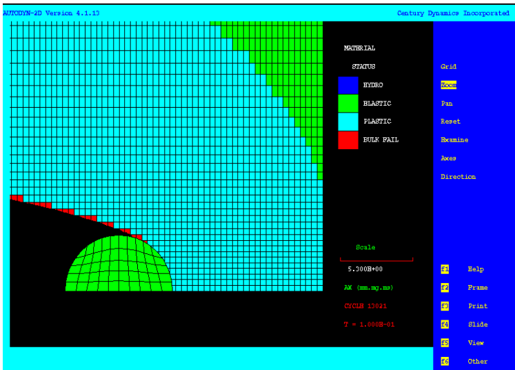
Figure 4.1 The grid of the target and projectile after 0.1 milli second.
