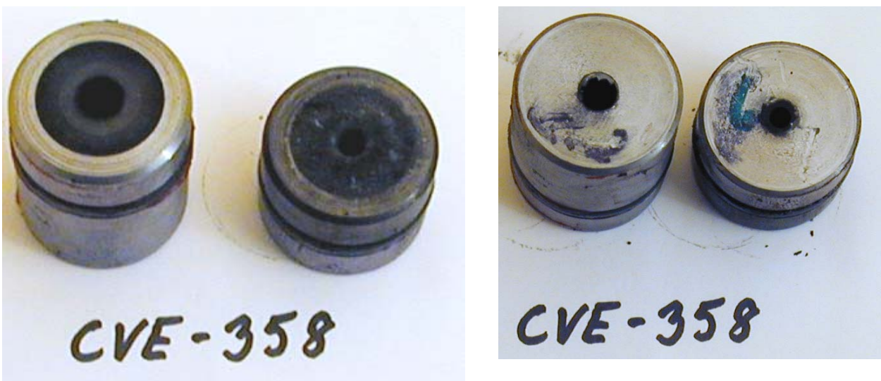
Figure 3.27 Pictures of entrance and exit side of both nozzles for the CVE-458 firing.
