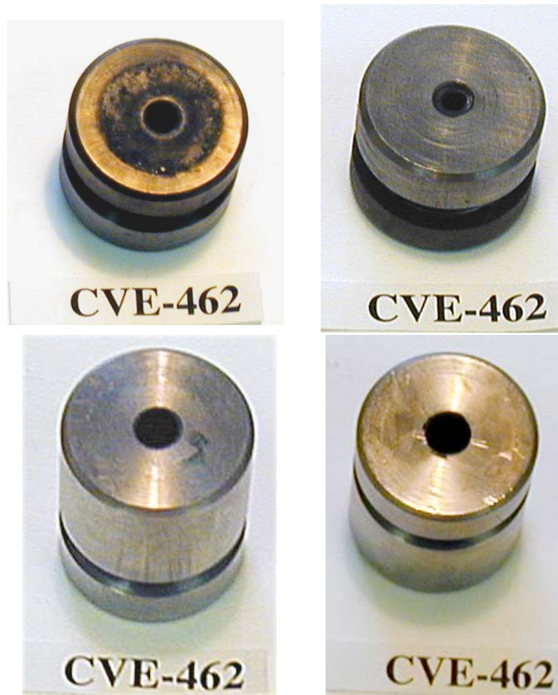
Figure 3.15 At the top pictures of inner nozzle for firing CVE-462 after firing and at the bottom pictures of the outer nozzle.
