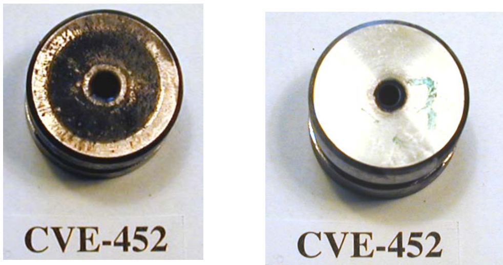
Figure 3.31 Pictures of the inner nozzle used in CVE-452 with CAB/RDX propellant after firing.
