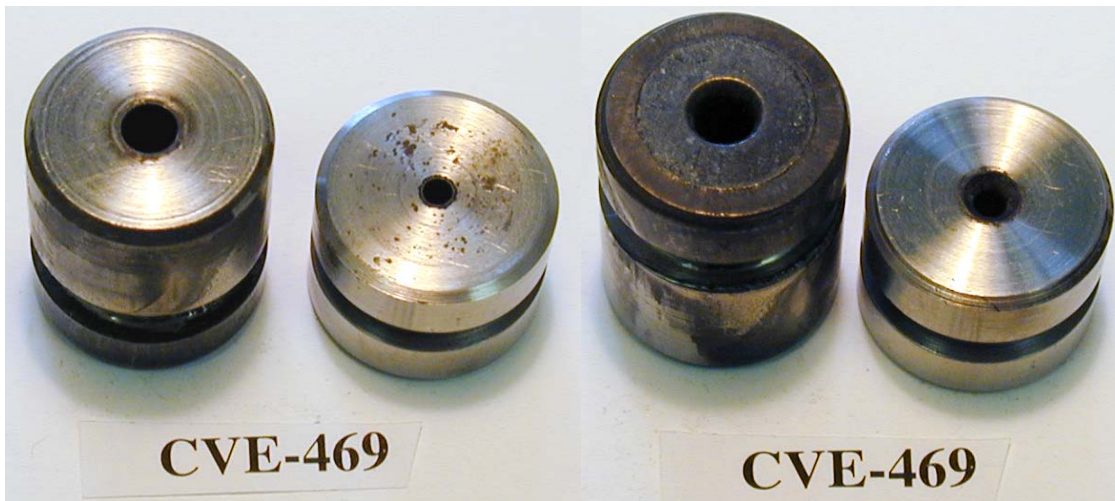
Figure 3.44 Pictures of the nozzles for firing CVE-469 having outer nozzle bore diameter of 2 mm.
