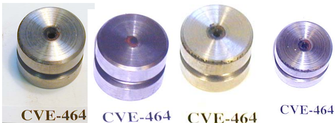
Figure 3.35 Pictures of the outer nozzle for firing CVE-464 with PB Clermont propellant.
