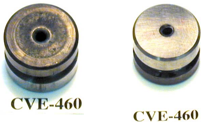
Figure 3.10 Picture of entrance and exit surface of the nozzle used for CVE-460 after firing.
