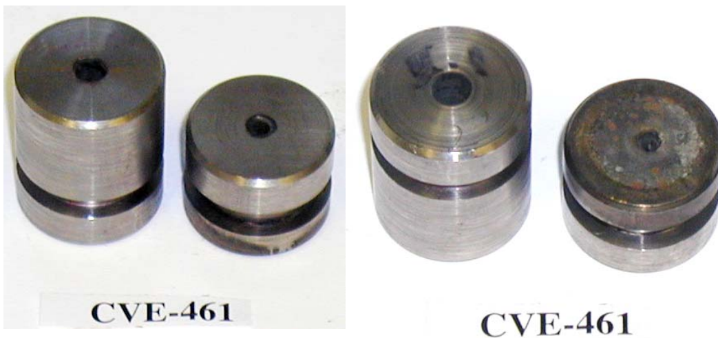
Figure 3.25 Pictures of entrance and exit side for the nozzles used in firing CVE-461.
