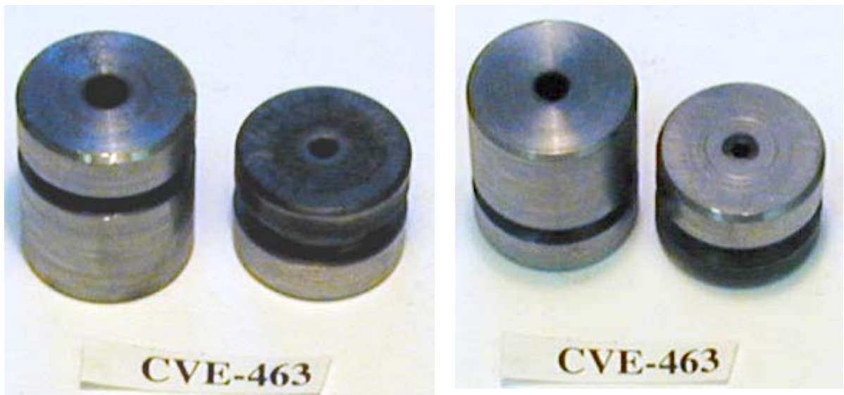
Figure 3.33 Pictures of both inner and outer nozzles entrance and exit sides after firing of CVE-463.
