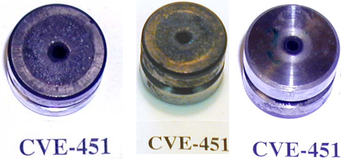
Figure 3.19 Pictures of the inner nozzle after firing with 12.7 mm PB Clermont propellant.
