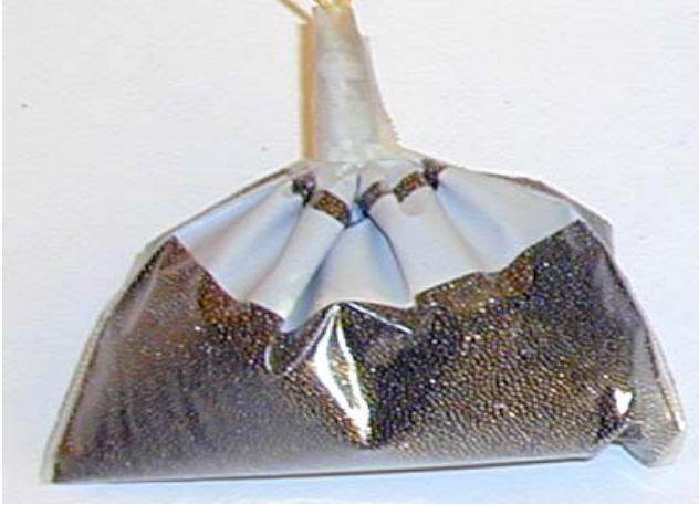
Figure 3.18 Picture of the ball powder grains in the plastic bag before testing.
