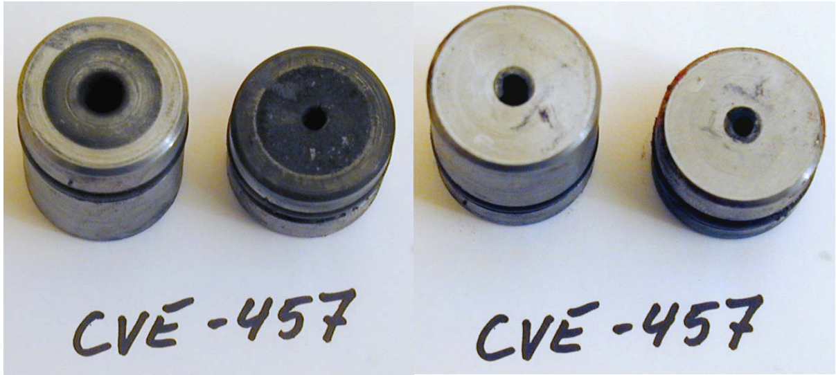
Figure 3.23 Pictures of entrance and exit side of the nozzle used in firing CVE-457.
