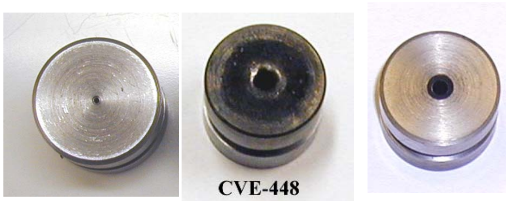
Figure 3.12 The nozzle before and after firing, in the center inlet and to right outlet.
