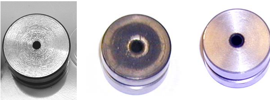
Figure 3.4 Pictures of inner nozzle (3 mm) before firing to the left, after firing inlet surface in the middle and outlet to the right.
