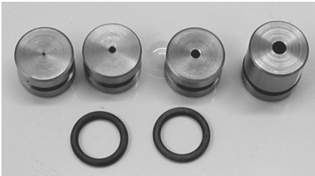
Figure 2.4 Picture of three inner nozzles with different bore diameter and the outer nozzle.
