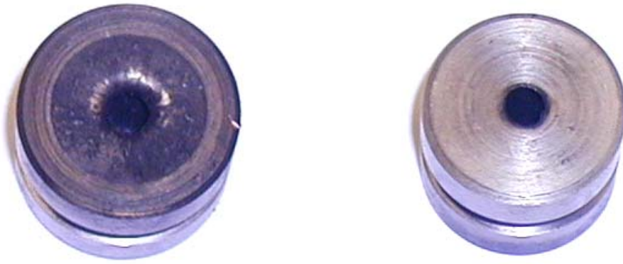
Figure 3.3 Pictures of 4.58 mm nozzle after firing, inlet surface to the left and outlet to the right.
