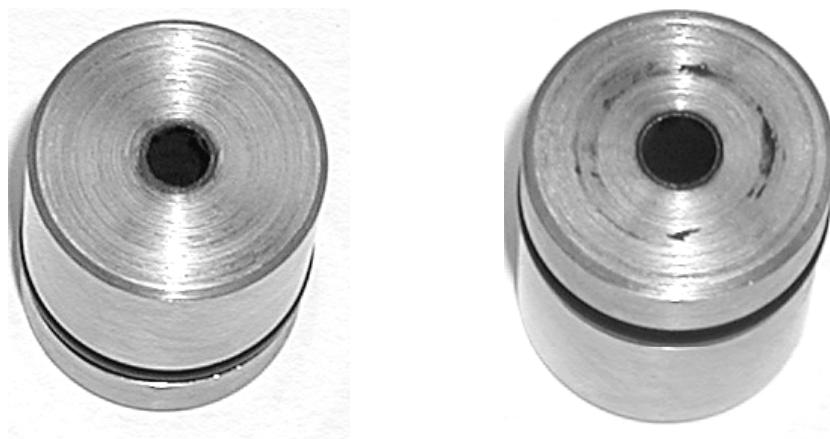
Figure 3.13 Picture of outer nozzle, inlet to the left and outlet to the right.
