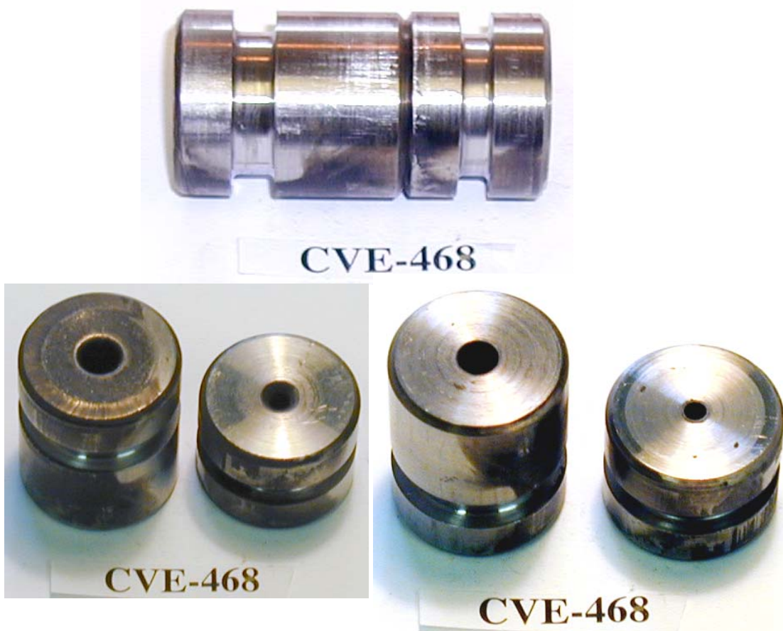
Figure 3.43 Pictures of the nozzles for firing CVE-468 having outer nozzle bore diameter of 2 mm.
