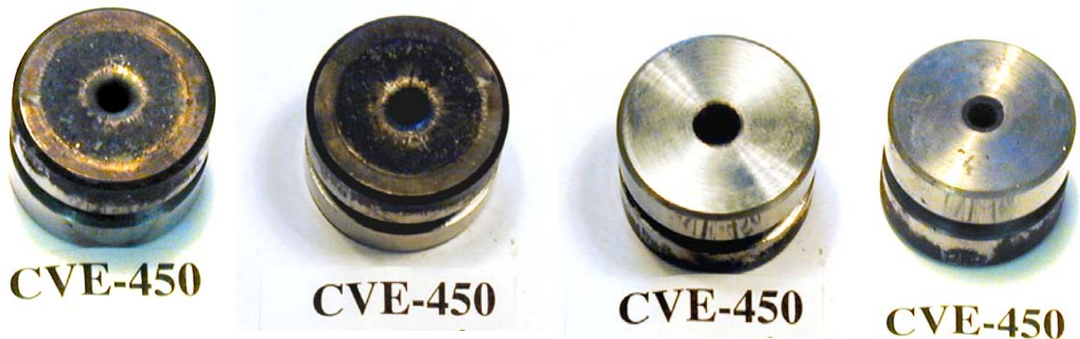
Figure 3.6 Inner nozzle after firing, left side inlet right side outlet.
