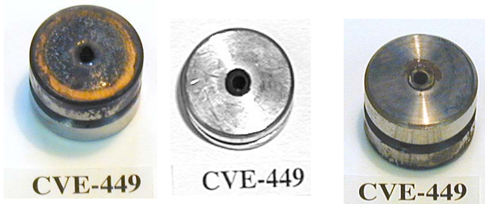
Figure 3.14 Inner nozzle after firing, left side inlet in the middle and right side outlet.
