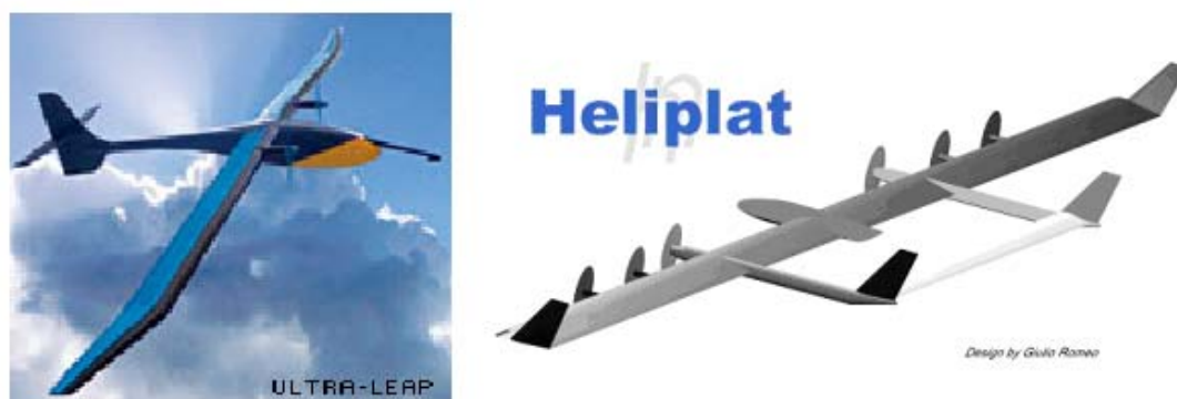
Figure 5.9 Left: The Boeing and DARPA ULTRA-LEAP. Right: The European Helinet Consortium Heliplat. These are examples of High Altitude Platform (HAP) projects that are exploring extreme altitude (30km) and extreme endurance (several weeks to several months).
