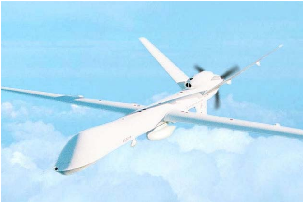
Figure 5.1 General Atomics Aeronautical Systems (GA ASI) Altair. The Altair is being used by NASA as a testbed for operations in controlled airspace. It is a modified version of the GA ASI Predator B (Photo: GA ASI).
