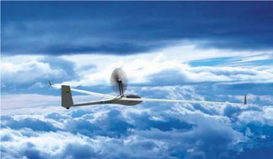
Figure 5.8 The Lange Flugzeugbau Antares is a very high performance electrically powered sailplane. The engine folds into the fuselage behind the cockpit when it is not in use. Sailplanes using this engine configuration must use the engine in “bursts” to gain altitude when needed. Flight with the engine deployed is very inefficient. When the engine is stowed, such sailplanes achieve extremely efficient flight (Photo: Lange Flugzeugbau).
