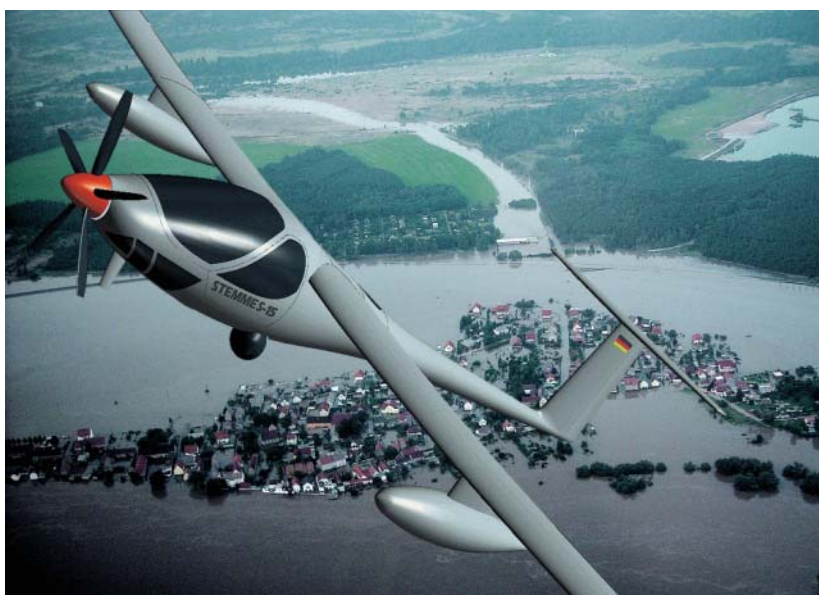
Figure 5.7 The Stemme Flugzeugbau S15-8 motorglider is currently under development for surveillance and communications relay missions. Stemme aims to have it certified for manned operation within two to three years, and for unmanned operation after that (Photo: Stemme).
