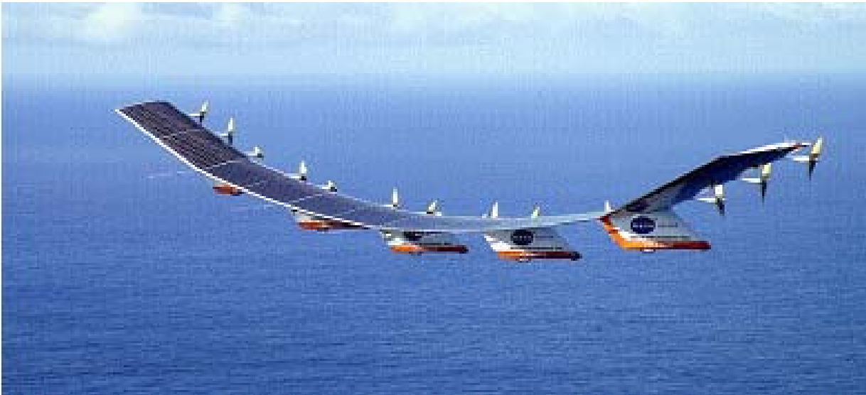
Figure 5.10 The Aerovironment and NASA Helios is the first to demonstrate that 30km altitude flight for many months is within reach. (Photo: NASA)
