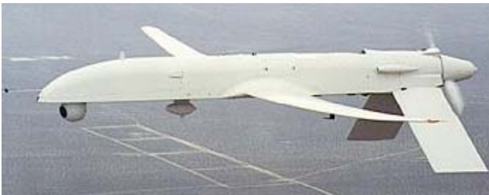
Figure 5.4 General Atomics Aeronautical Systems (GA ASI) I-GNAT has an exceptional endurance of 52 hours, which is possible due to a relatively light payload (90kg). It is suitable for a number of communications missions. The Predator is based on the I-GNAT, but sacrifices some endurance for a heavier payload and a large SATCOM bulge (Photo: GA ASI).
