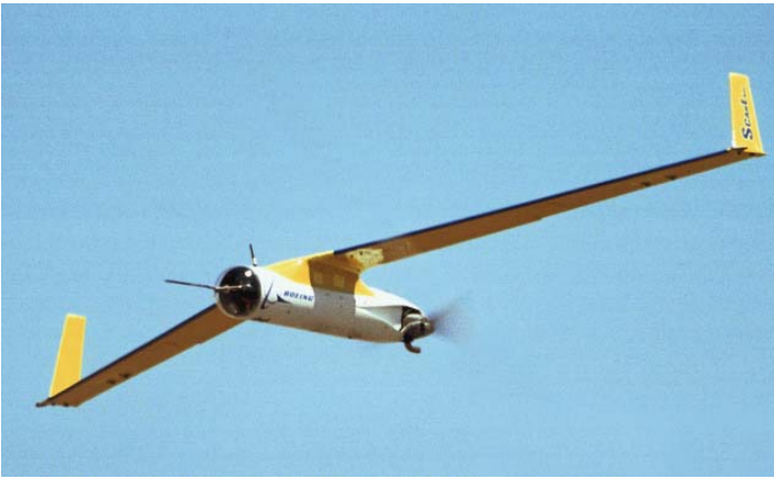
Figure 5.5 The Insitu Group SeaScan is a good example of a LALE UAV, capable of multi-day missions with light payloads. (Photo: The Insitu Group)
