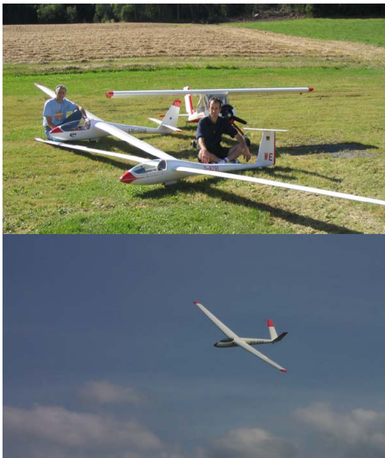
Figure 5.1 Examples of large-scale model sailplanes. Top picture in the foreground: an ASW 15b in scale 1:1,25, with a wingspan of 6m and a total weight of 19 kg. Bottom picture: a 1:2,5 scale SHK of 6,8m wingspan and 25 kg total weight. The towplane (a Wilga, 1:2,5 scale also) is in the background in the top picture.
