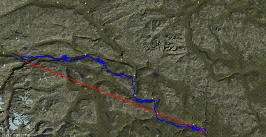
Figure 3.1 Flight-path optimisation performed in the “Silent Wings” flight simulator developed by Simula Research Laboratory AS in Oslo, Norway. The blue (wiggly) line represents the path that maximises the probability of lift given the current weather forecast. At some points along the path, thermals or strong slope lift is exploited to gain extra altitude (shown as “knots” on the blue line).
