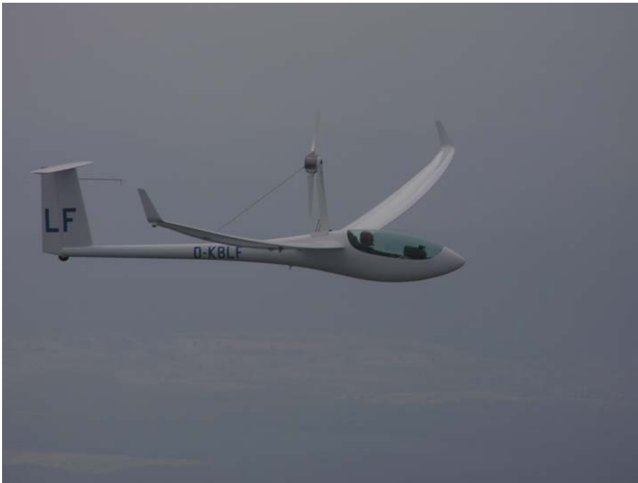
Figure 5.3 The Lange Flugzeugbau Antares prototype in flight with the engine deployed (Photo courtesy of Lange Flugzeugbau, Germany).
