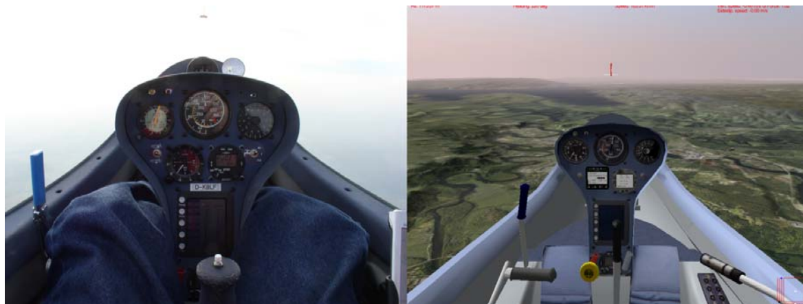
Figure 6.1 Remote piloting in the Silent Wings simulator developed by Simula Research Laboratory AS, Oslo, Norway. The picture on the left was taken from the pilot position in dense fog. The picture on the right shows the simulated view, based on a detailed terrain model and aircraft telemetry data.
