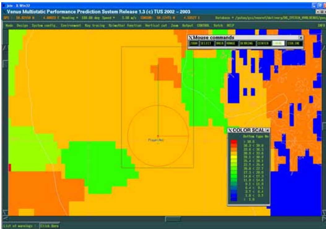
Figure 3.4 Sediment type available in VENUS corresponding to second experiment area (green – coarse sand, light brown – mud, dark brown – sandy mud)
