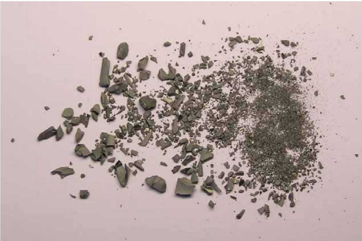
Figure 2.2: The hardmetal test specimen after fracture.
