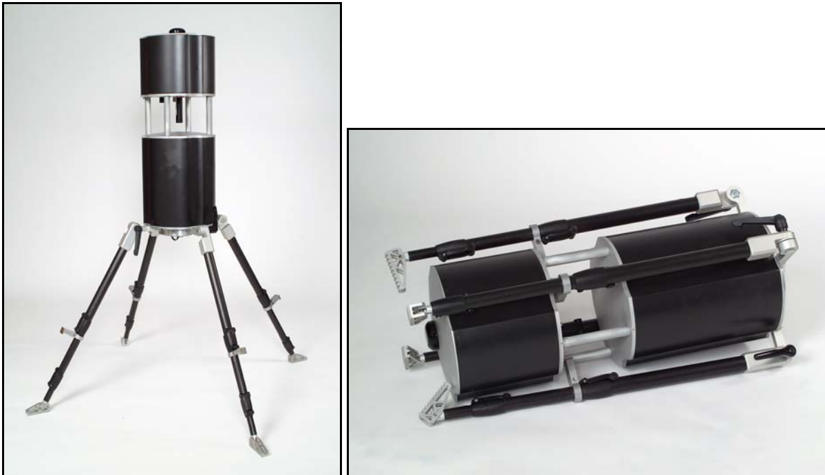
Figure 2.1 The newly designed CATSS unit called Templum during operation (left) and transport (right). The Templum is made from carbon (black) and aluminium (gray)
