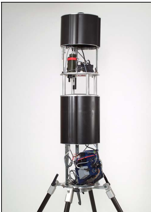
Figure 2.2 The Templum opened to have access to the upper (detector) and lower (computer) compartments. The computer in the lower compartment is unfolded
