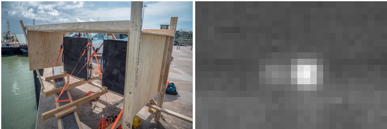
Figure 2. Blackbodies at Stokes Hill Wharf. Left: The blackbodies were mounted side-by-side on the pier. A provisional “sun screen” kept the blackbodies out of direct sunlight. Right: Crop from the IRCAM LW image of the two blackbodies. The temperatures were T_{cold} = 34.8^\circ\text{C} and T_{hot} = 48.6^\circ\text{C} .
