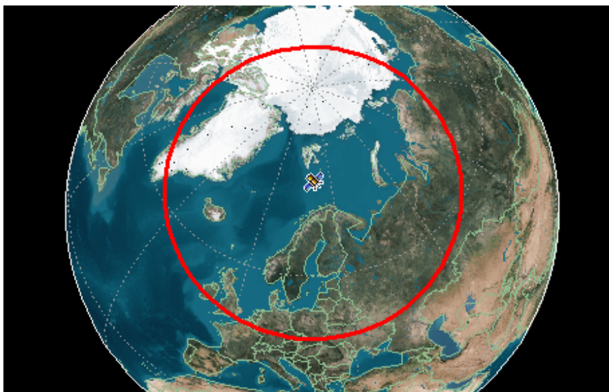
Figure 1.1 A space-based concept for AIS reception. The red circle indicates the AIS sensor's field of view to horizon from 600 km altitude.
