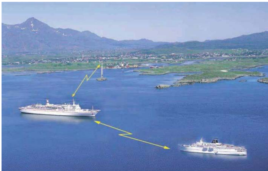
Figure 2.1 The AIS ship-to-ship and ship-to-shore concept. (Courtesy of Kongsberg Seatex, Norway).
