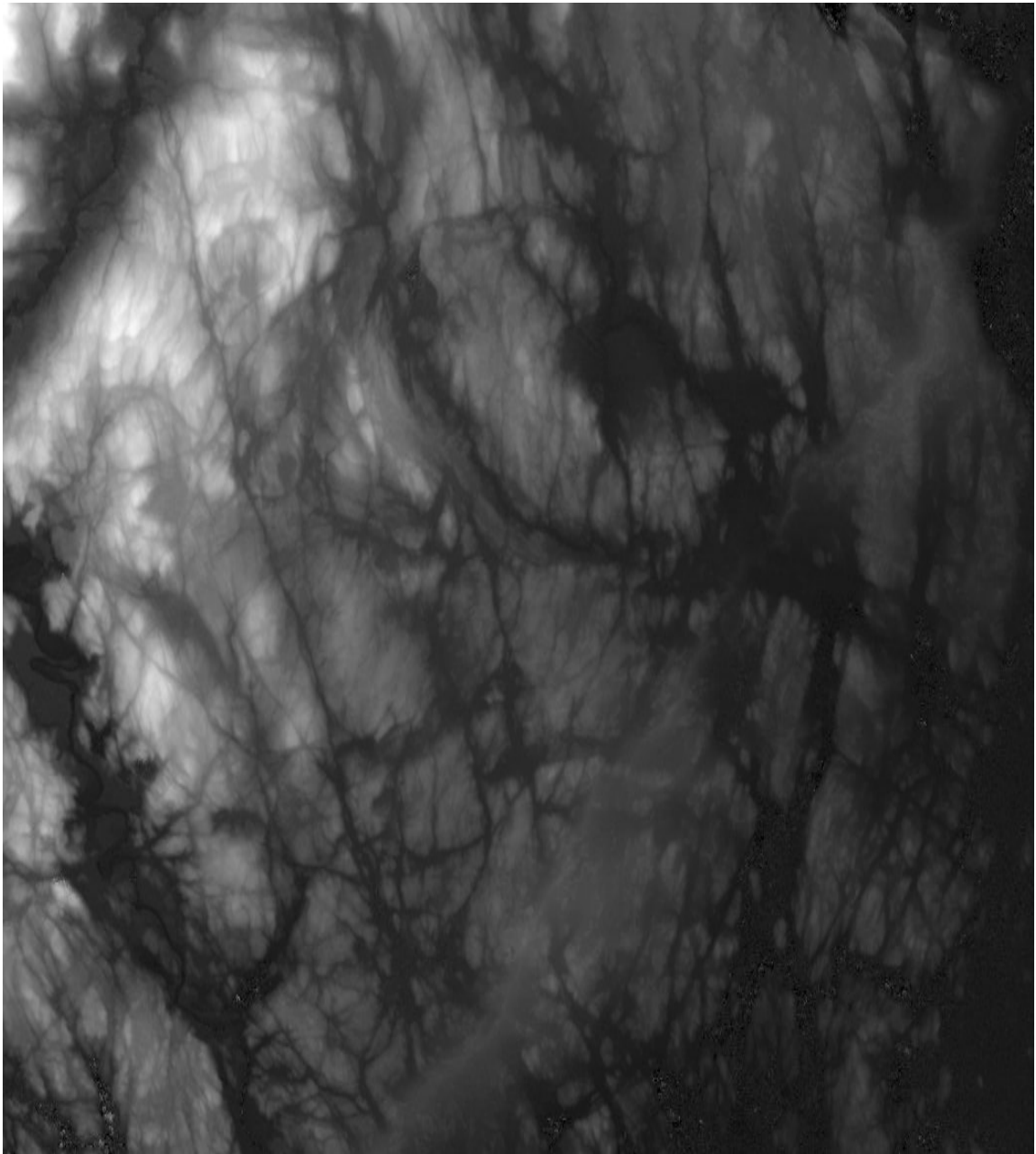
Figure 7.1 SRTM X-band DEM from the Vestfold test area. The above DEM covers an area of approximately 36.9 km (North) x 33.0 km (East). The present X-band DEM has a pixel spacing of approximately 30 m x 15 m in the Northing and Easting directions respectively. (© DLR 2003.)
