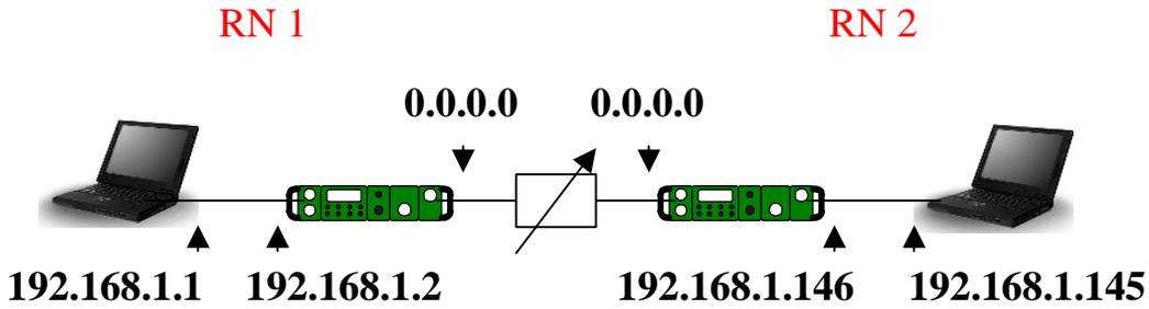
Figure 2 Radios in unconnected subnet using the IP bridging feature
