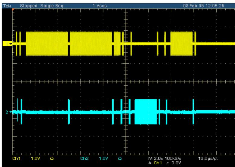
Figure 6 Signalling over-the-air when transmitting a 403 byte MMHS message using the IP LOS mode of the AN/PRC-117F. PDU-delay 150 ms, Cipher text, AUTO data rate, poor channel conditions
