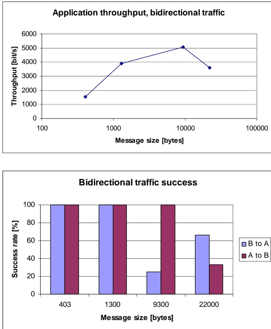
Figure 8 Bidirectional total throughput including the effect of lost messages (upper panel). Success rate of transferred messages (lower panel). Radio parameters: data rate AUTO, ARQ enabled. MMHS parameters: PDU-size 1024 byte, PDU-delay 1 s.
