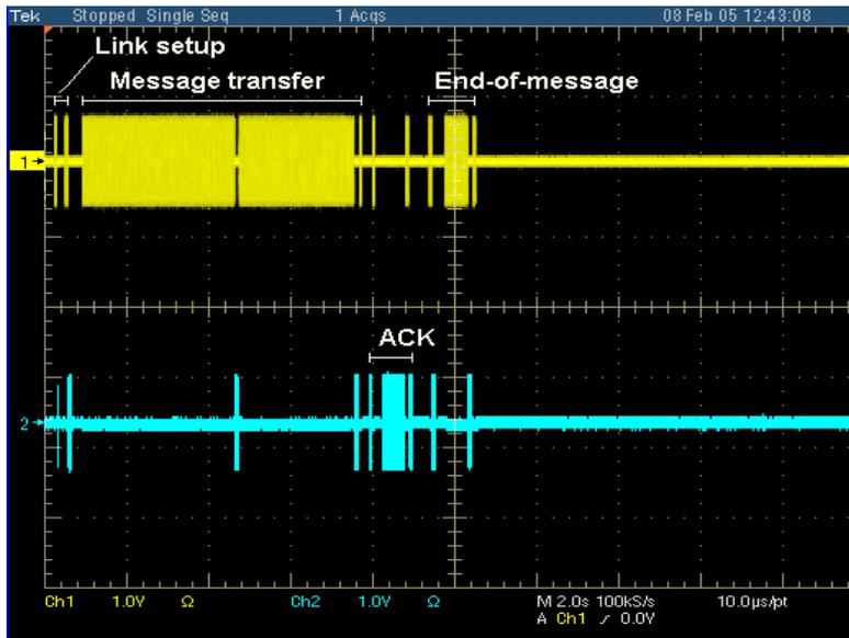
Figure 5 Signalling over-the-air when transmitting a 403 byte MMHS message using the IP LOS mode of the AN/PRC-117F. PDU-delay 150 ms, Plain text, AUTO data rate, poor channel conditions
