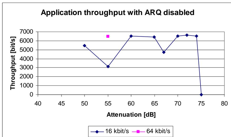
Figure 10 Application throughput for a 22 kbyte message using the non-ARQ data link protocol. MMHS parameters: PDU-size 1024 bytes, PDU-delay 1 s.
