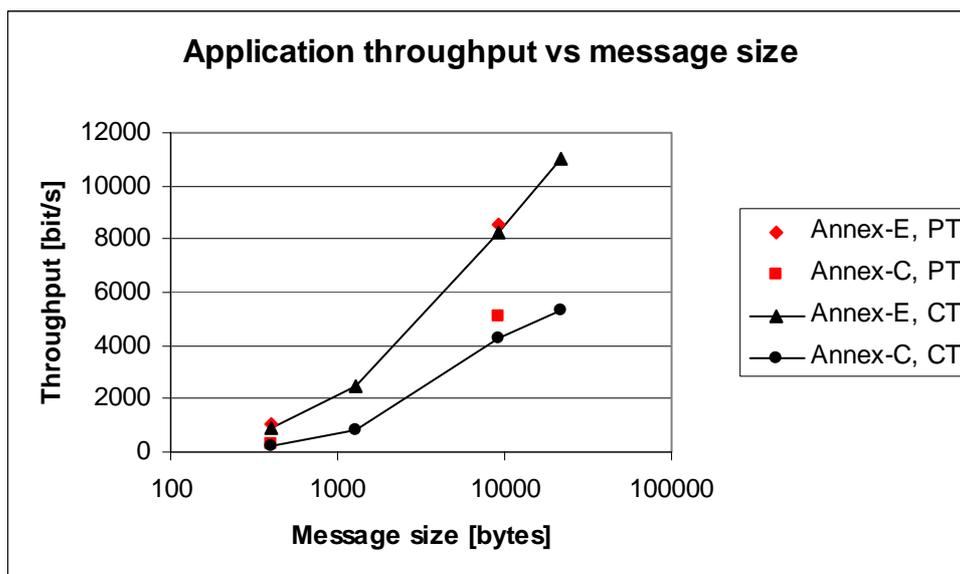
Figure 7 Application throughput (unidirectional) versus message size for S4406 Annex C and E in plain and cipher text mode, respectively. Radio parameters: data rate AUTO, ARQ enabled. MMHS parameters: PDU-size 1024 byte, PDU-delay 0.5 s. Ideal channel.
