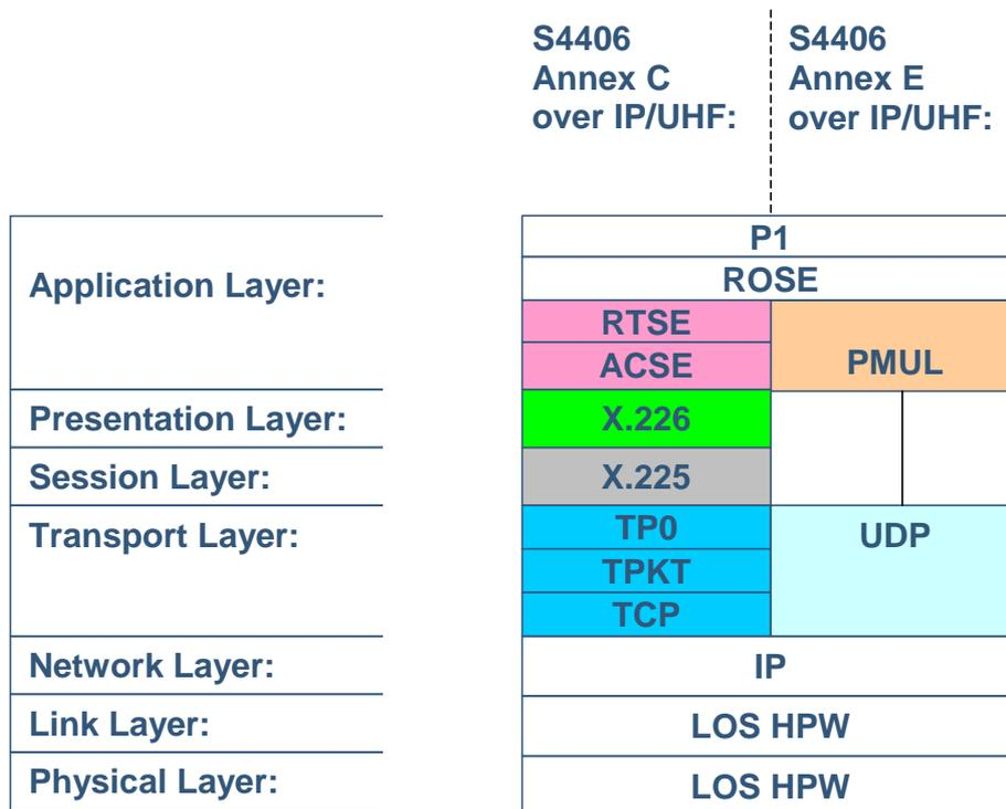
Figure 1 Protocol stack of MMHS (S4406) using IP over the LOS HPW (AN/PRC-117F)
