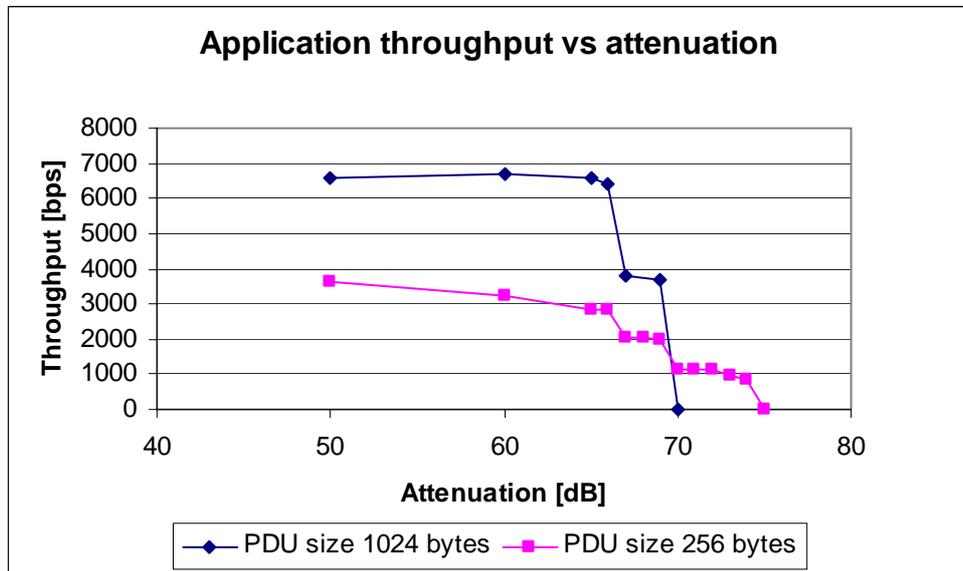
*Figure 9 Application throughput versus attenuation for different PDU-sizes. Message transmitted: 22 kbyte. Radio parameters: data rate AUTO, ARQ enabled. MMHS parameters: For PDU-size 1024 byte, the PDU-delay is 1 s. For PDU-size 256 byte, the PDU-delay is 0.25 s*
