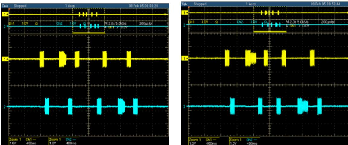
Figure 4 Traffic over-the-air when transmitting a single Ping with the data rate of the radio set to AUTO. Good channel conditions (left), medium channel conditions (right)
