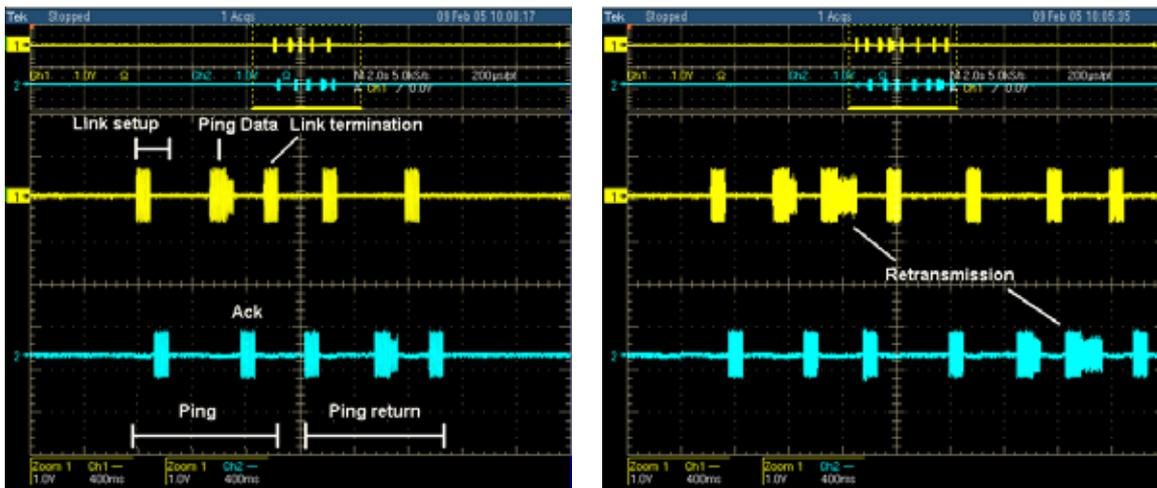
Figure 3 Traffic over-the-air when transmitting a single Ping with the data rate of the radio set to 64 kbit/s. Good channel conditions (left), medium channel conditions (right)
