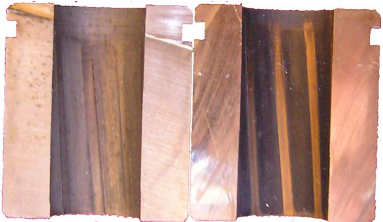
Figure 3.14: Gun barrel used with varnish at projectile (left) and without varnish (right).
