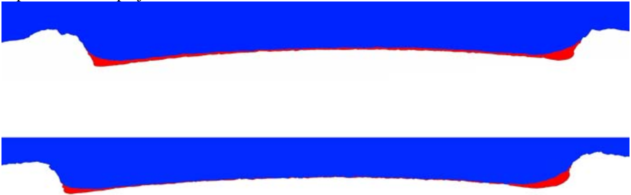
Figure 3.11: Comparing lands from the shot series with varnish (lower) and without (upper).
