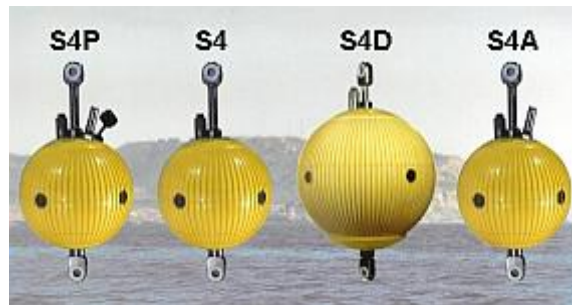
Figure 5.6 Electromagnetic current meters from InterOcean Systems Inc.
