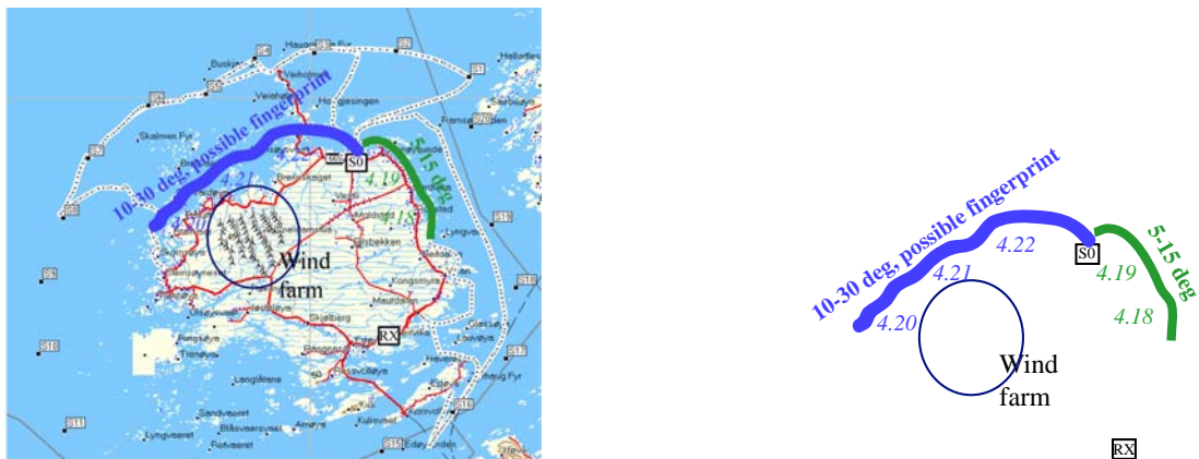
Figure 4.33 Summarizing figure for measurements at 9.991 MHz. With (left) and without (right) map overlay. Boldface comments refer to phase fluctuations (in units of electrical phase difference), while italics refer to figure numbers in this report.
