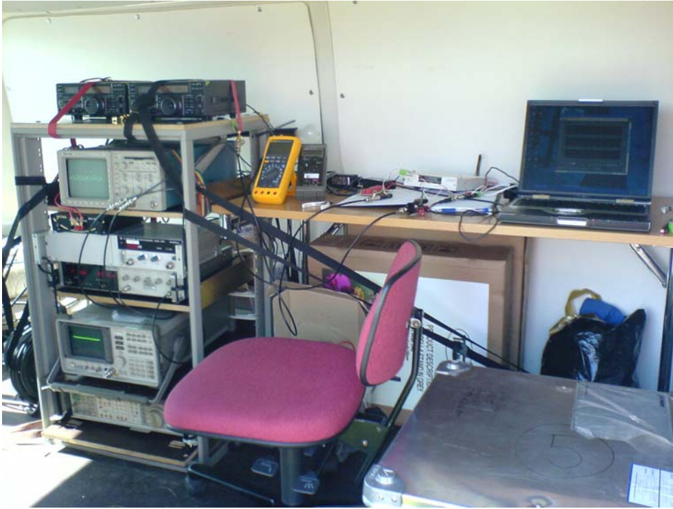
Figure 4.5 Receiver measurement equipment, mounted in the back of a Volkswagen Transporter and powered by a Honda generator.
