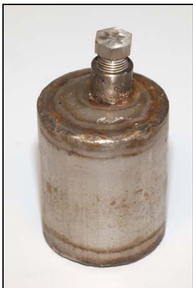
Figure 1.1 Steel container where VX was stored for more than 40 years
