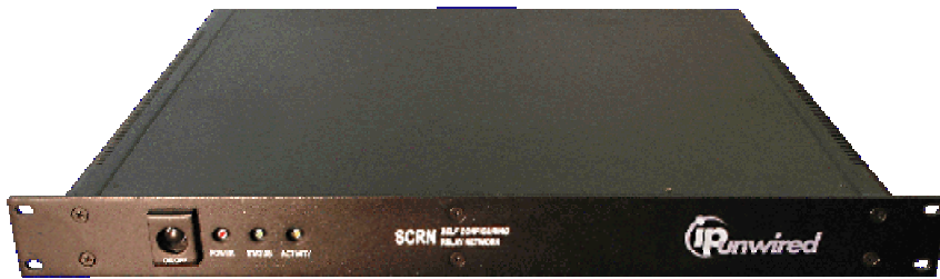
Figure 2.1 SNR reconfigurable 1 st generation hardware (controller, modem or HF channel emulator)
