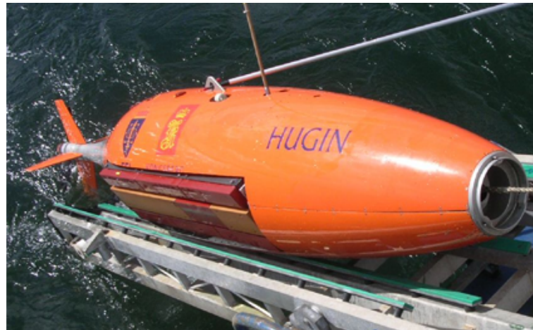
Figure 1.1: SENSOTEK SAS on the HUGIN I AUV during recovery.
