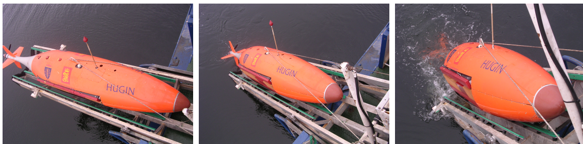
Figure 2.2: HUGIN I AUV with SENSOTEK during launch from M/S Simrad Echo on the very first test March 17, 2005.
