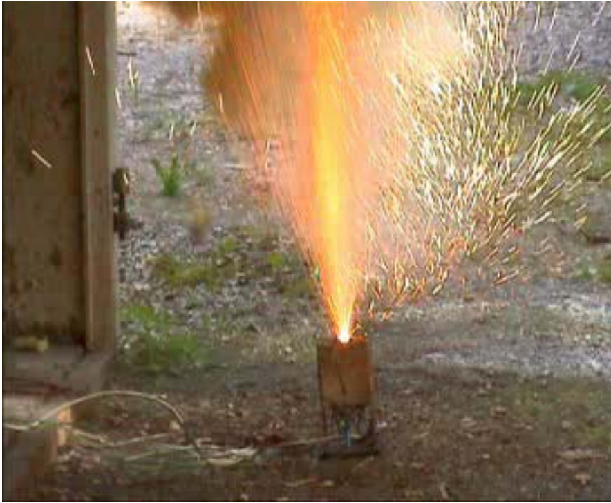
Figure 5.15 Enlarged frame of Picture 012.tif showing violent venting of CSC cell at 50% SOC.
