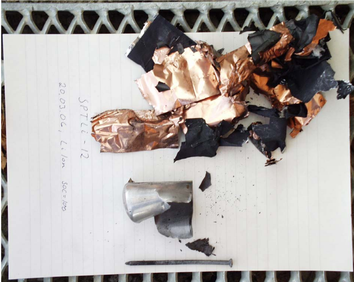
Figure 5.5 Lithium Ion D-cell after nail penetration at 100% SOC and room temperature. The cell exploded after 111 seconds with flames.
