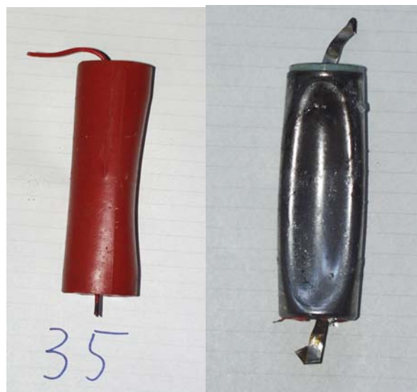
Figure 5.11 Cell after the experiment in fig 5.5. Left with potting, right after the removal of the potting.
