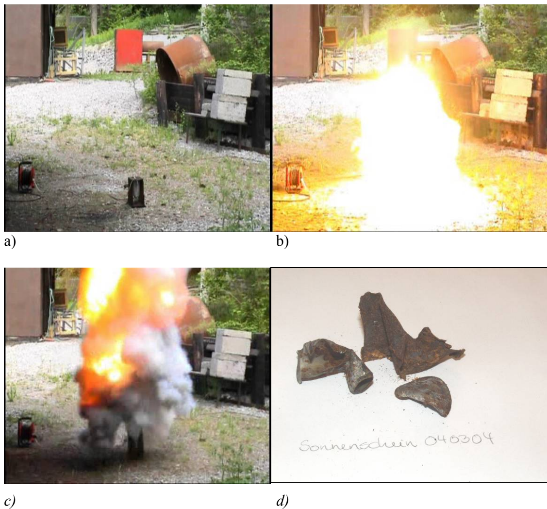
Figure 5.19 Heating of SL-780 Li/SOCl 2 bobbin cell. a – c shows frames from the video, it is 40 ms between each frame. Picture d shows remains from the cell after the explosion.
