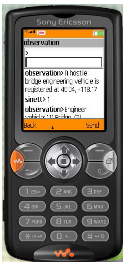
Figure 4.7 IM client on an emulated mobile phone in dialog with the IM-bot
