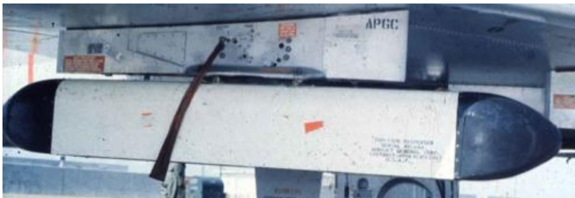
Figure 5.2 A typical dispenser unit; the American SUU-13[3]
