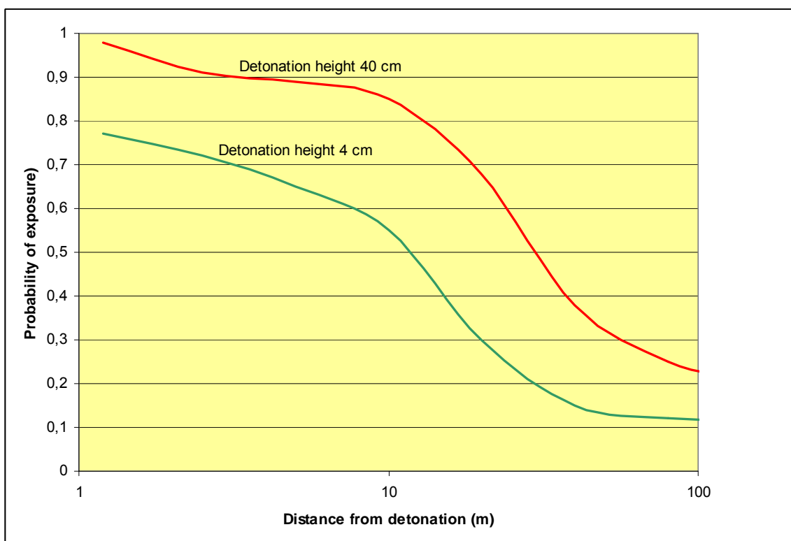
Figure 7.1 The effect of rugged terrain. The figure shows the probability of exposure of a prone soldier from a detonation height of 4 cm and 40 cm. (Example: A soldier located 10 m away from the detonation is only 55% exposed to a DPICM detonating 4 cm above ground)
