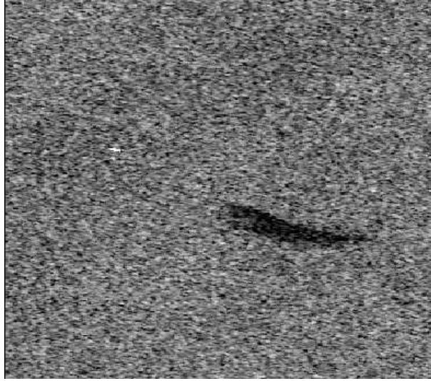
Figure 1.3: RADARSAT-1 SCN near range mode subscene (19th of July 2003) containing an oil slick look-alike (at 55,47N, 12,28E) detected as oil spill by Kongsberg Satellite Services AS (KSAT), QinetiQ and Norwegian Computing Centre (NR). The size of the subscene is 394 \times 359 pixels. ©CSA/KSAT 2004.
