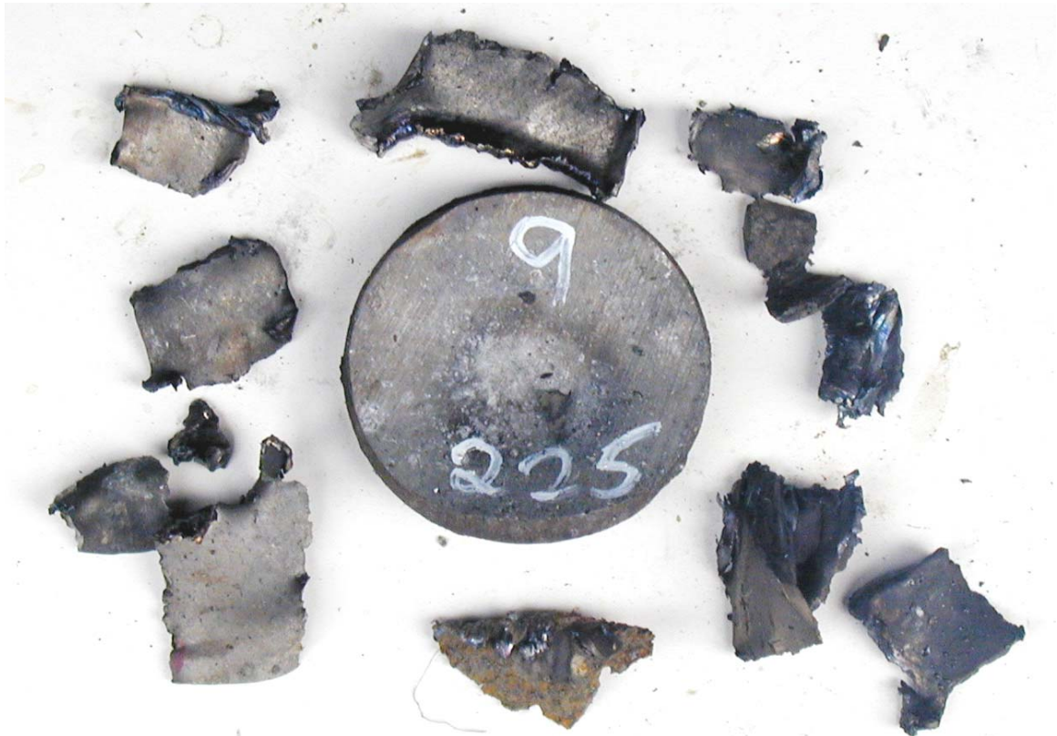
Figure 3.9 Shot No 9, tube No 9, barrier 225 cards, no reaction.
