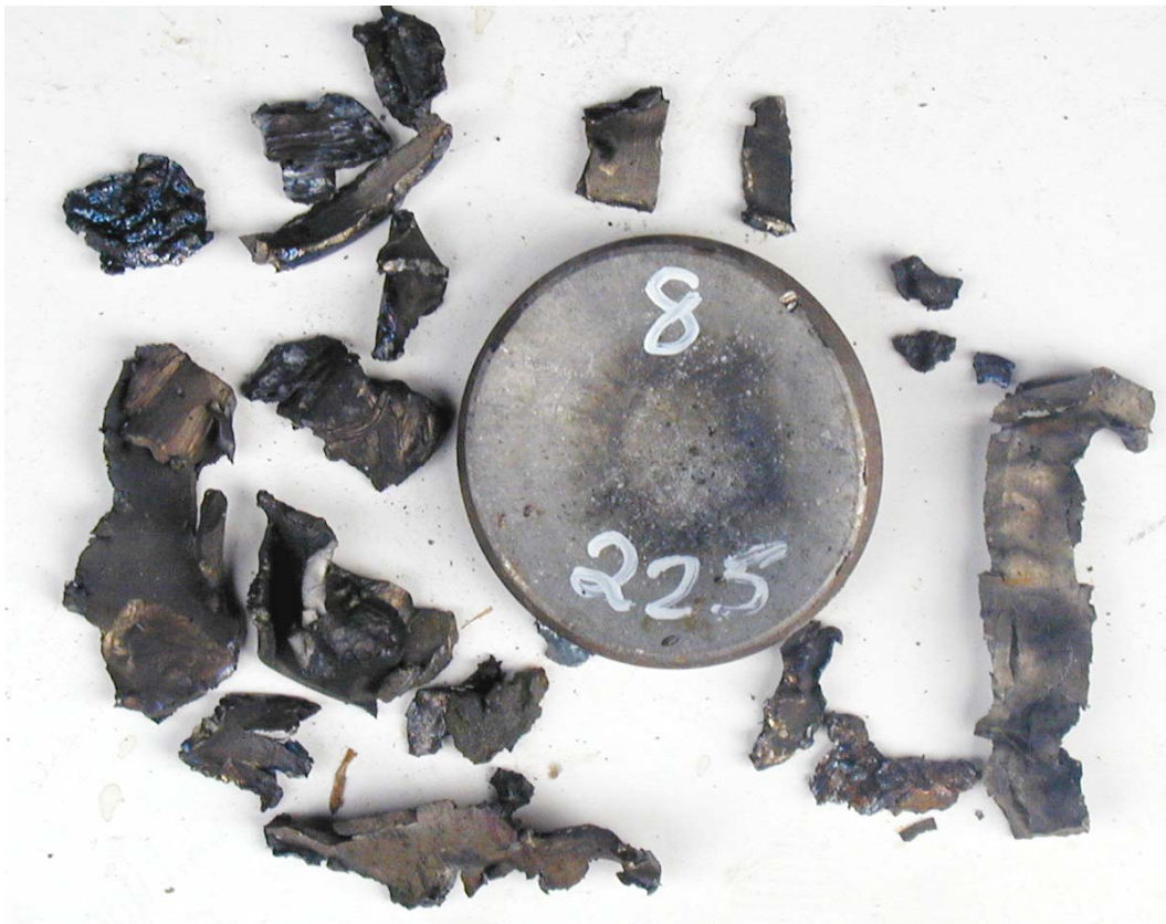
Figure 3.8 Shot No 8, tube No 8, barrier 225 cards, no reaction.
