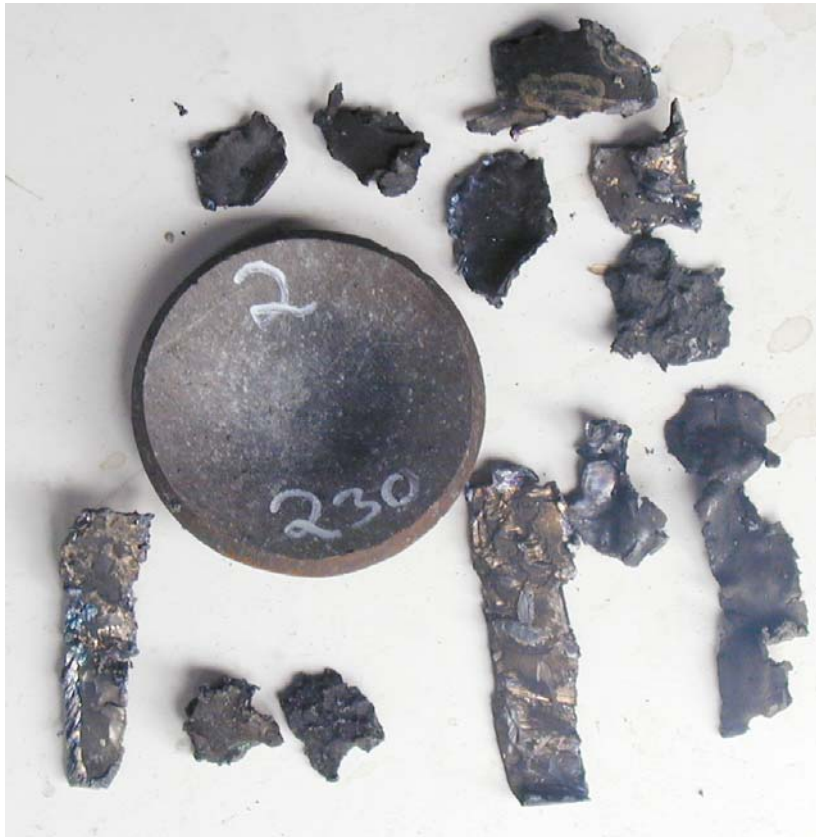
Figure 3.2 Shot No 2, tube No 2, barrier thickness 230 cards, no reaction.
