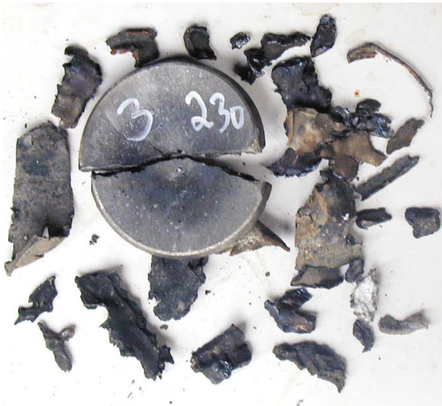
Figure 3.3 Shot No 3, tube No 3, barrier 230 cards, no reaction.
