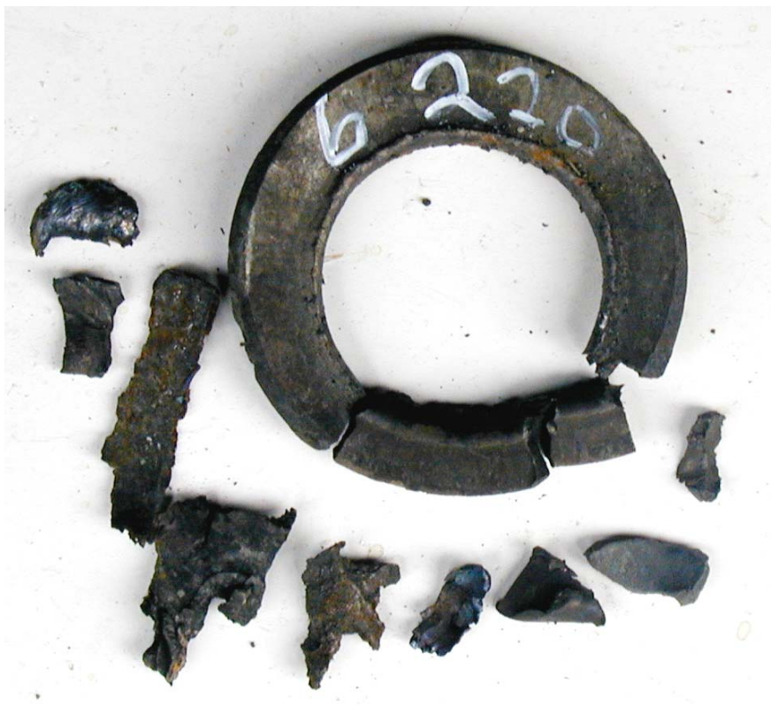
Figure 3.6 Shot No 6, tube No 6, barrier 220 cards, detonation.
