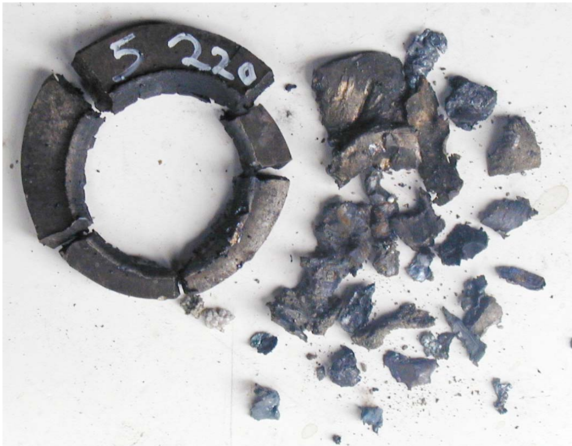
Figure 3.5 Shot No 5, tube No 5, barrier 220 cards, detonation.
