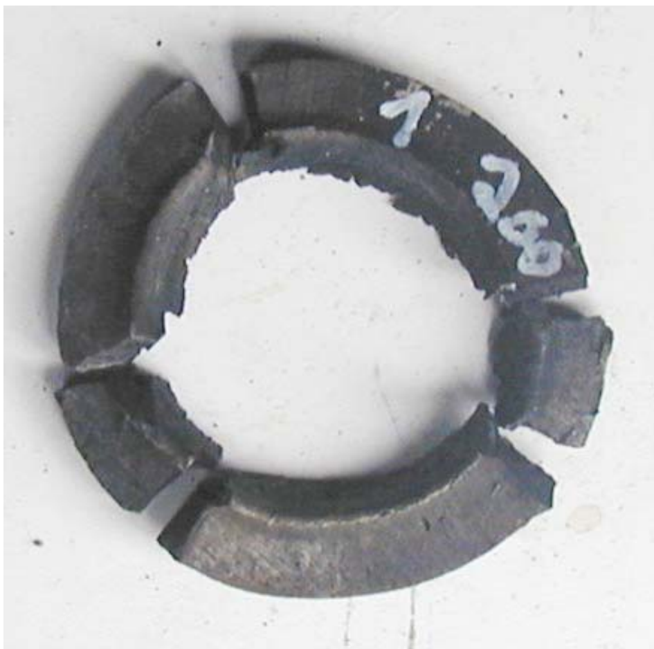
Figure 3.1 Shot No 1, tube No 1, barrier thickness 200 cards, detonation.
