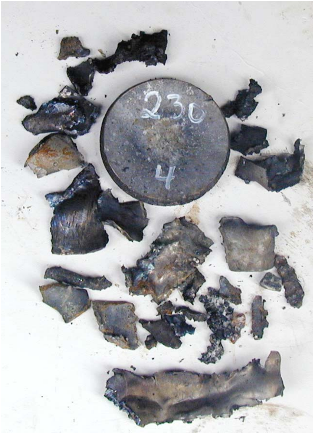
Figure 3.4 Shot No 4, tube No 4, barrier 230 cards, no reaction.
