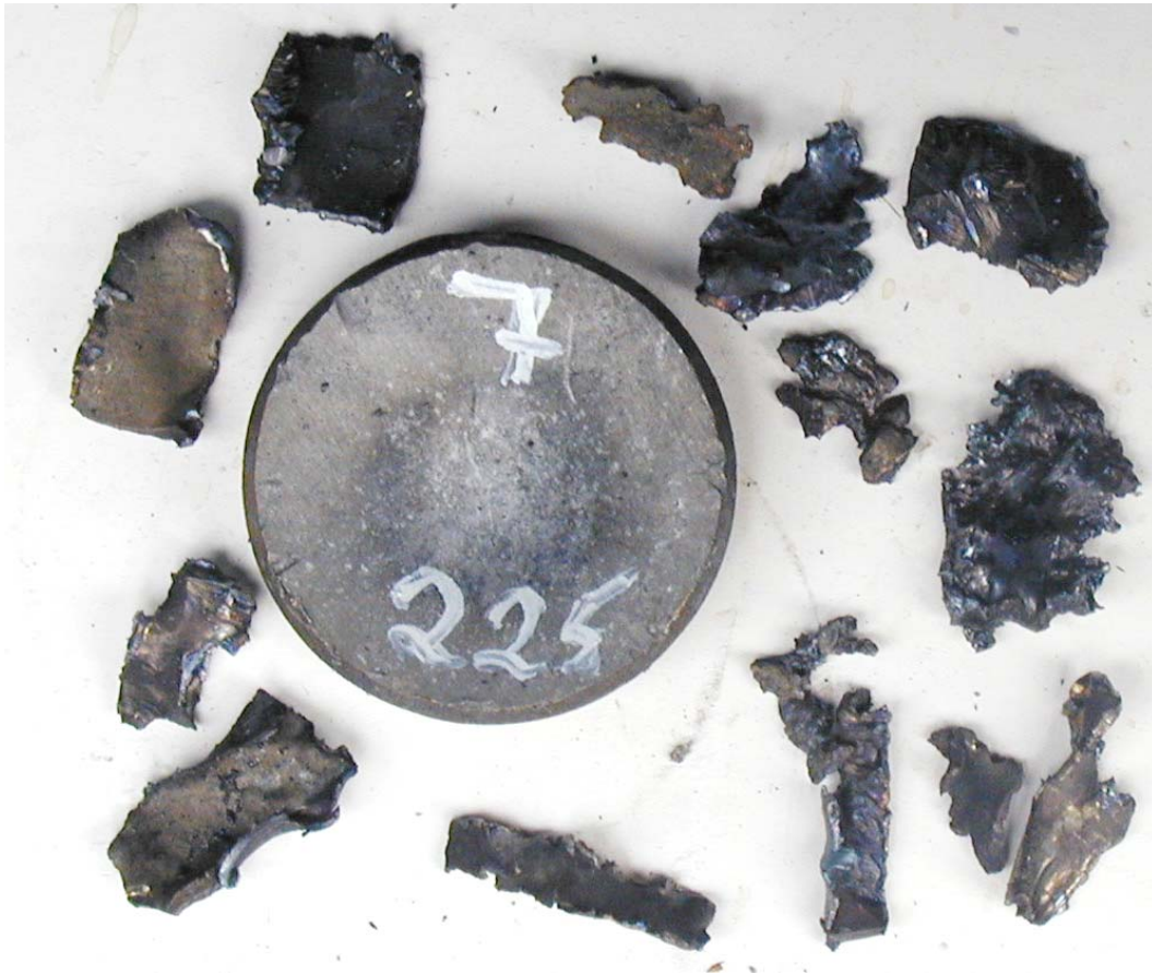
Figure 3.7 Shot No 7, tube No 7, barrier 225 cards, no reaction.
