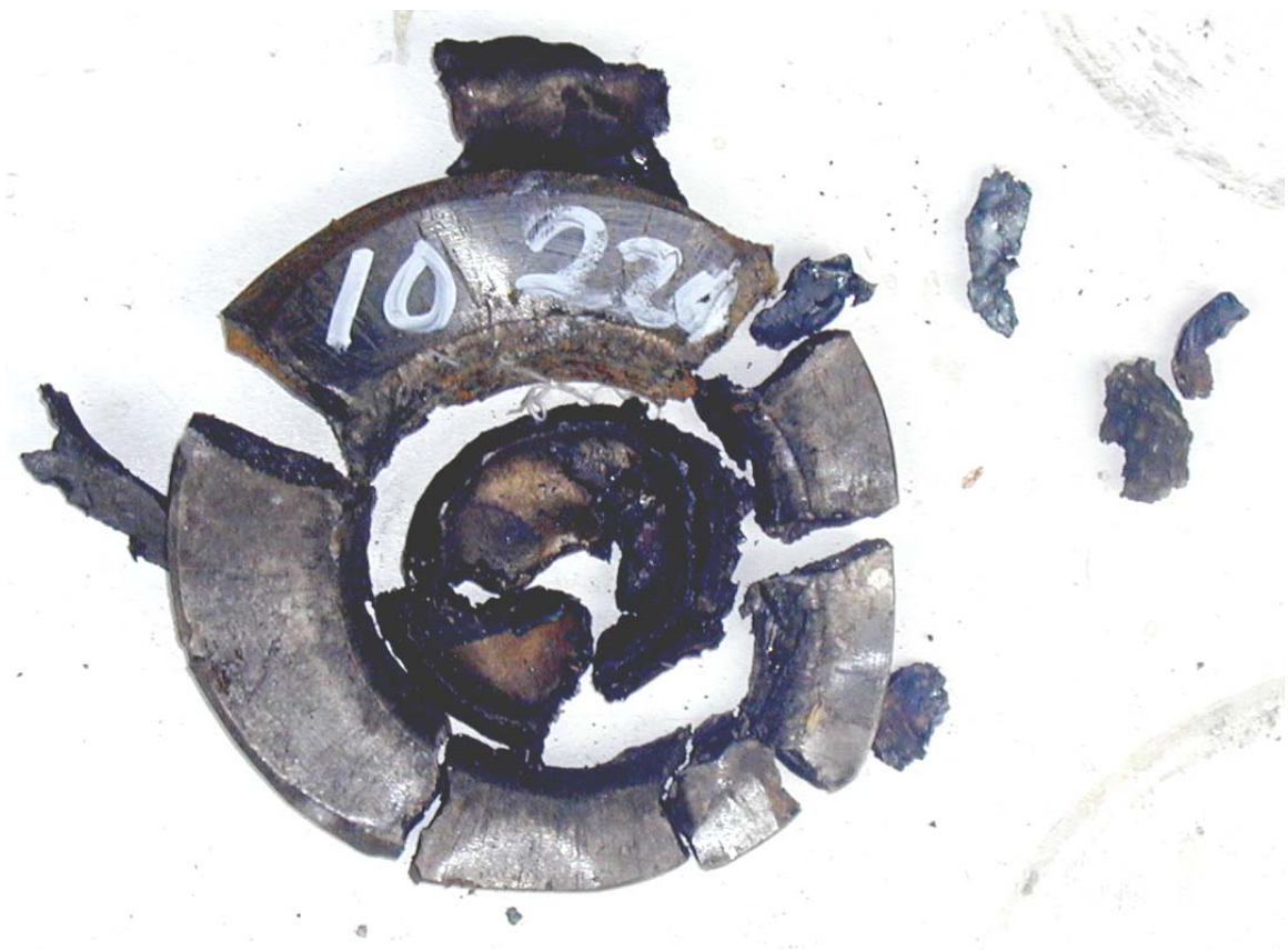
Figure 3.10 Shot No 10, tube No10, barrier 220 cards, detonation.
