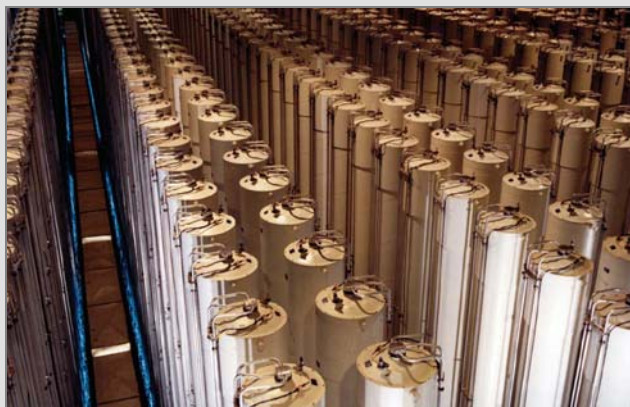
A small section of the Ohio centrifuge enrichment plant. A centrifuge is typically two to four meters tall. (Picture courtesy of U.S. Department of Energy.)
