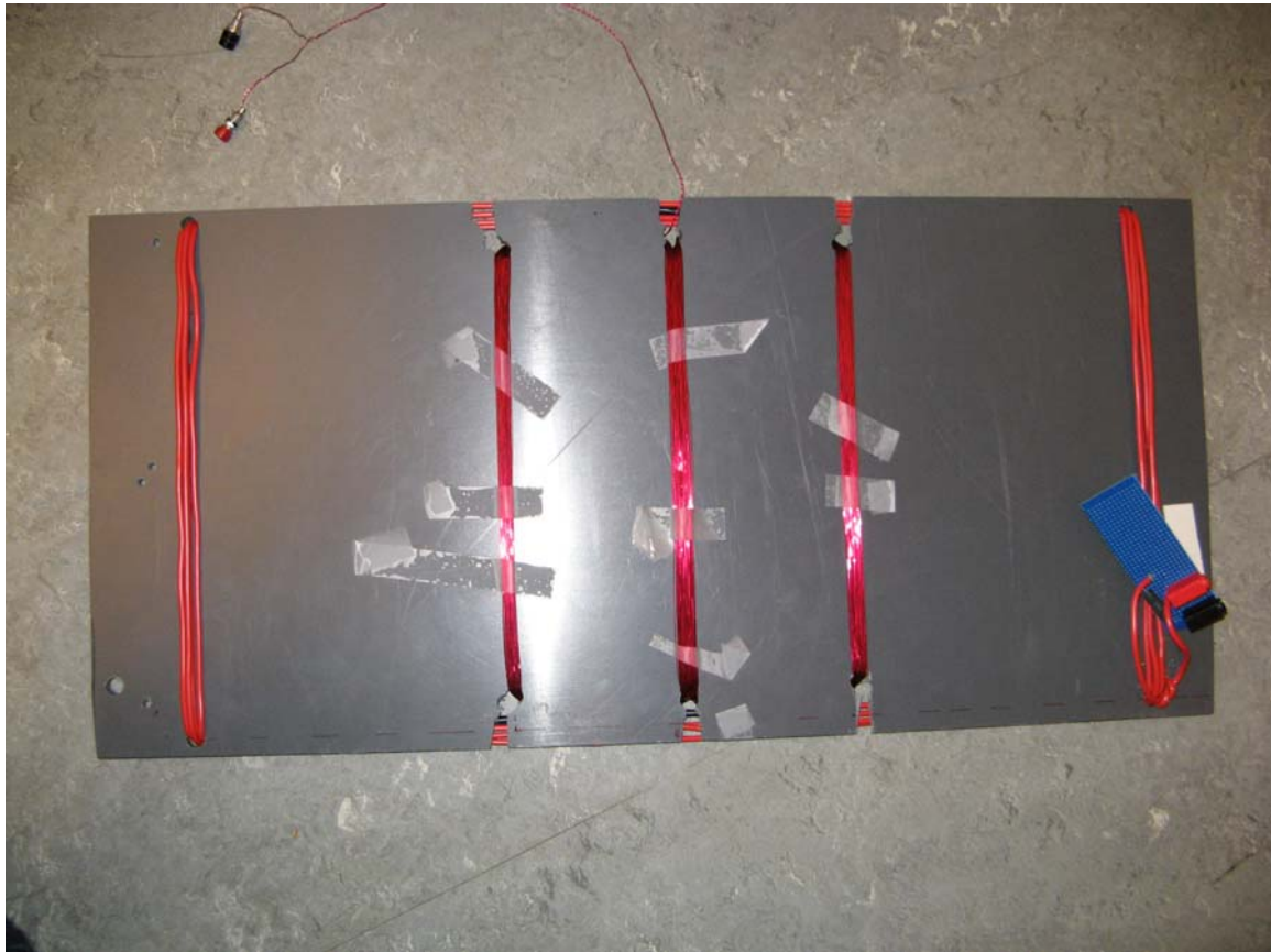
Figure 2.31 Preliminary experimental coils for IB concept Ia.
