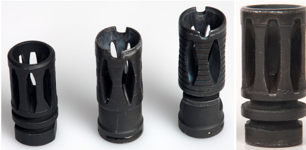
Figure 5.1 Flash suppressors. From the left: HK 416 N, AG3, HK 417, C8 SFW.
