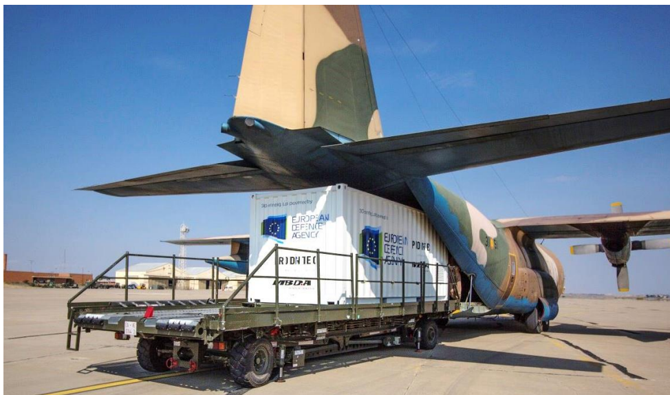
Figure 1.1 The EDA AM container is being put on a transport aircraft at the airbase in Zaragoza, Spain, and then airborne, to demonstrate the capabilities of in-field additive manufacturing. EDA ©. Source: European Defence Agency project on Additive Manufacturing (16.EDA.OP.144) lead by Fundación Prointec.
