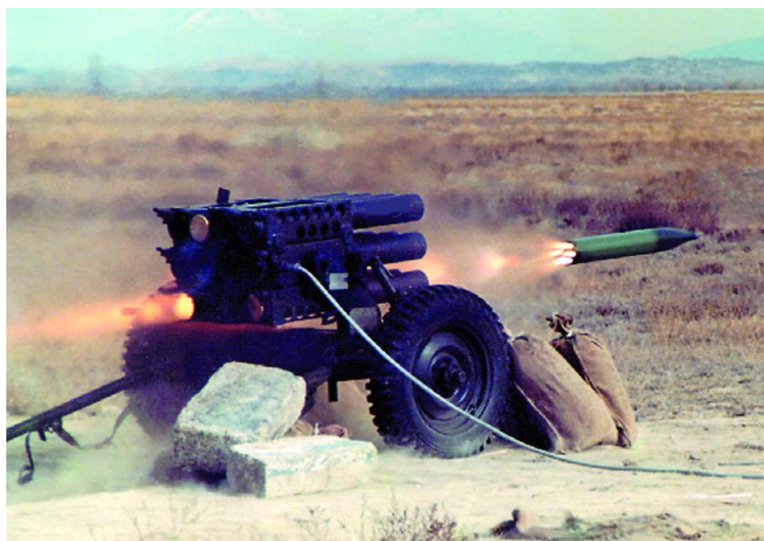
Figure 6.6 Test firing of a 107 mm spin stabilized rocket (MKEK)
