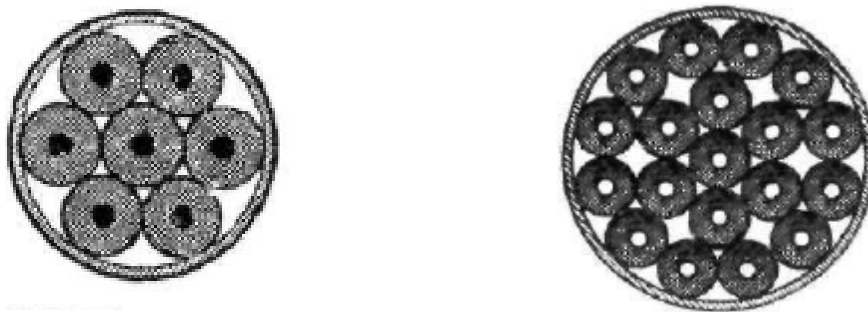
Figure 6.2 Cross sections of old propellant grain configurations (left - 140 mm; right - 240 mm)
