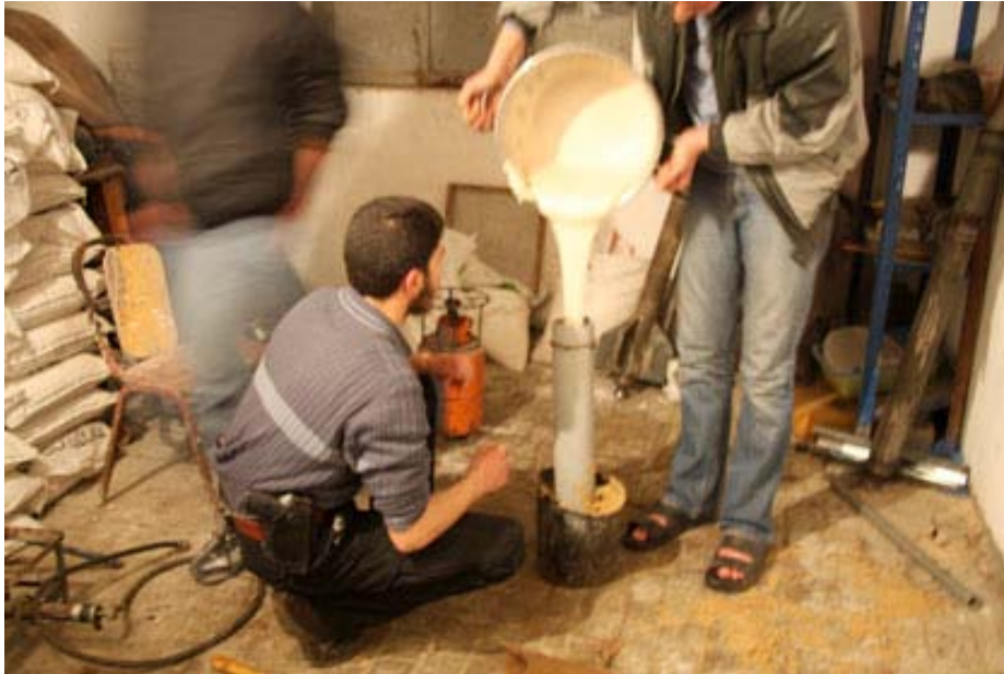
Figure 9.2 Improved rocket fuel being poured into a plastic casting container to cool and cure. The container is then cut away and the casting is placed inside the rocket. [26]
