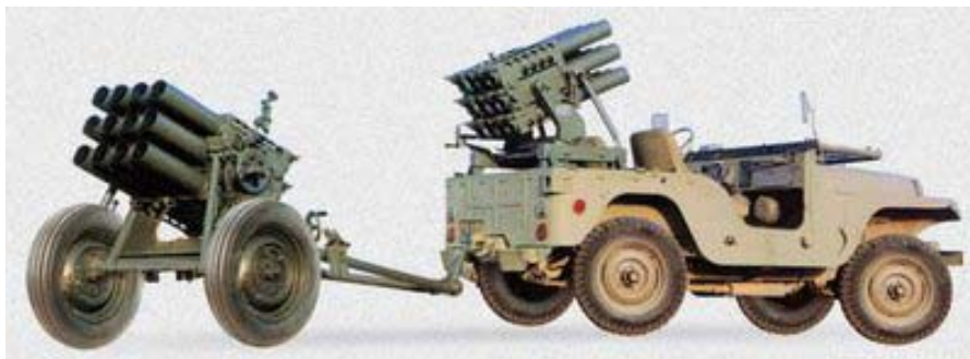
Figure 3.3 A 12-tubed towed system behind a light vehicle with the same system mounted on the vehicle
