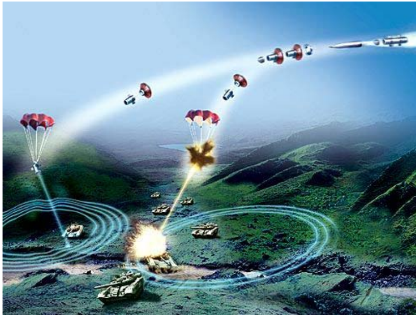
Figure 7.3 The search mode of a Sensor Fuzed Warhead
