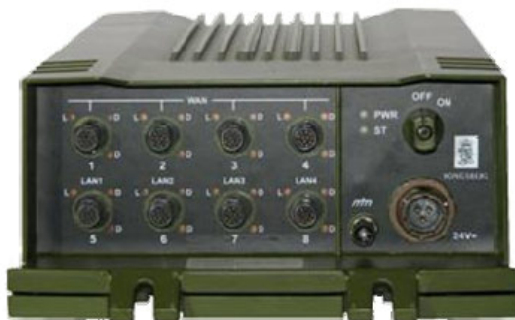
Figure 4.6 The Intelligent Tactical IP Router from KDA is based on a ruggedized PC/104 platform offering three ports for Ethernet or serial (RS232) connection, one port for Ethernet or serial (RS422)connections, and 4 ports for Ethernet connections only.
