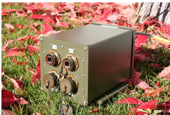
Figure 4.2 The Intelligent Tactical IP Router designed by Thales is based on a ruggedized PC/104 platform offering four Ethernet ports, two serial ports, one X.25 port and two USB ports
