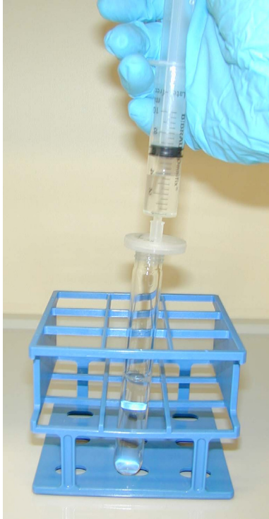
Figure 2.1 Illustration of the filtration procedure with a syringe membrane filter, (0.45 µm pore size).
