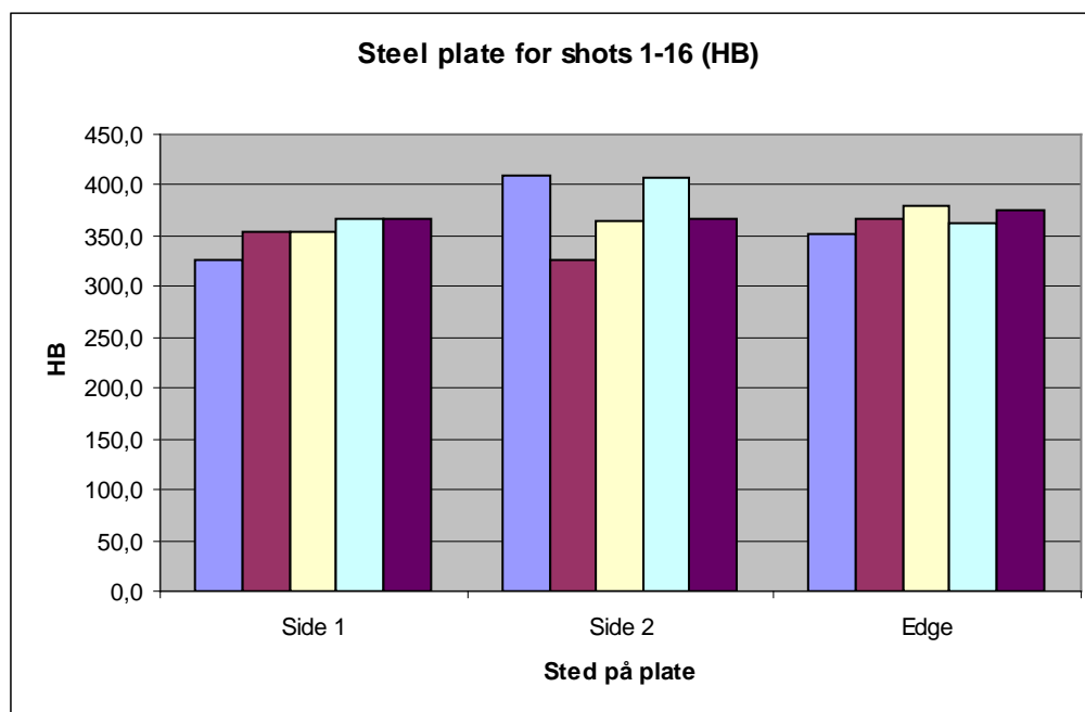
Figure A.1 Hardness measurement for steel plate used for shots 1-16 in the yaw experiments. Both sides and the edge were measured.
