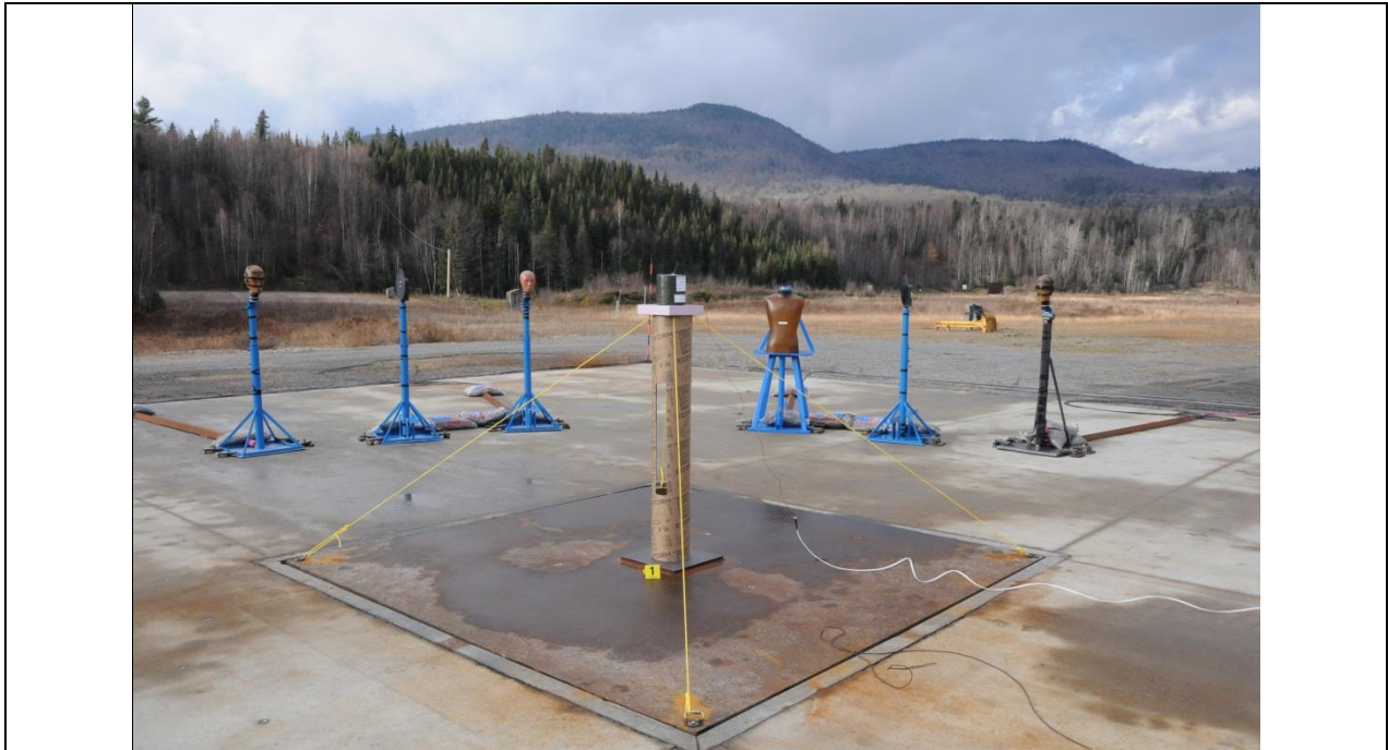
Figure 7. A example of full-scale explosive test set-up simulating the above-ground detonation of a large charge, centrally located relative to a series of target.
