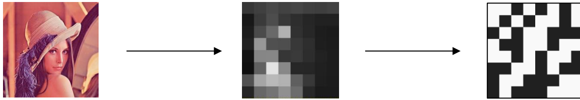
Figure 11: Process of transforming image into a minor representation (middle) and into a 64-bit perceptual hash (right).
