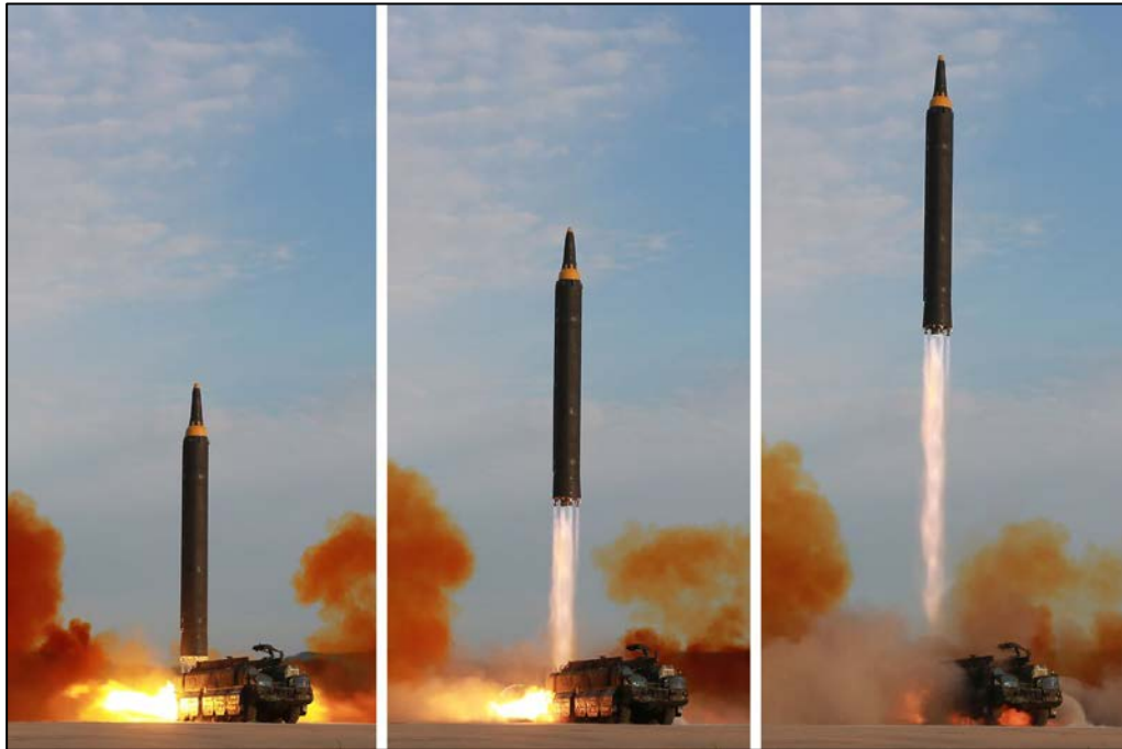
Figure 4.7 Launch of a Hwasong-12 IRBM sometime in 2017 (image released 16 September 2017). The plumes from the main engine and four vernier engines (probably of the SS-N-6/Hwasong-10 type) are clearly visible. Credit: AFP.
